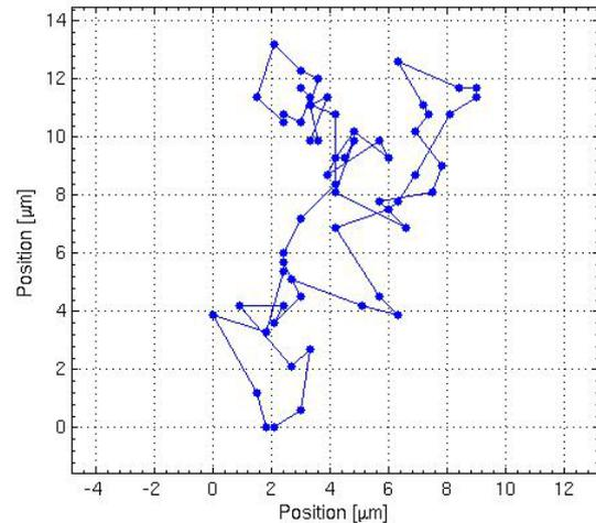
Fig. 4: Typical trajectory of a Brownian motion. The particle was 300nm in diameter, time between points is 0.5s
