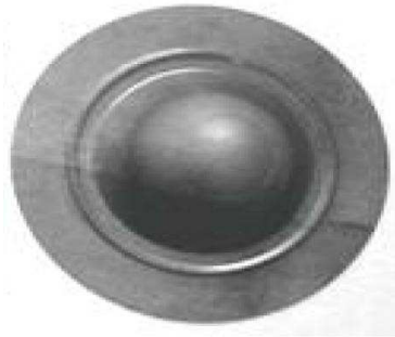
Fig. 2: The experimentally deformed shape of sheet metal
