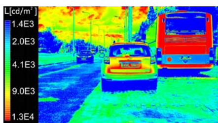
Fig. 4 Environment luminance distribution [cd/m 2 ]. daytime, summer, vehicle directly illuminated by the sun (changed range of luminance visualization).
