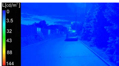
Fig. 5 Environment luminance distribution [cd/m 2 ]. Nighttime, summer, vehicle illuminated with street lanterns.
