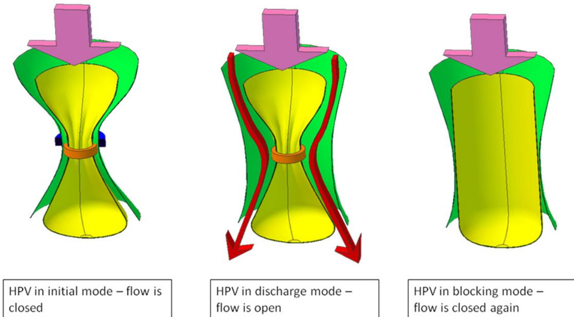
Figure 10: The HPV sequence of operation (beginning from left hand side)
