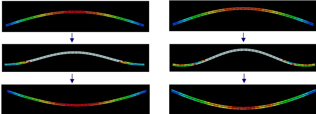
Figure 7: Snap-through of three-layer arch caused by induced deformation of the layers:
