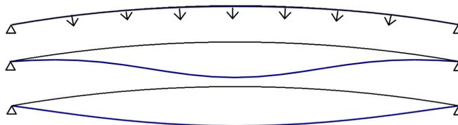
Figure 6: Snap-through of arch caused by distributed pressure loading: a) state just before snap-through, b) snap-through, c) state just after snap-through
