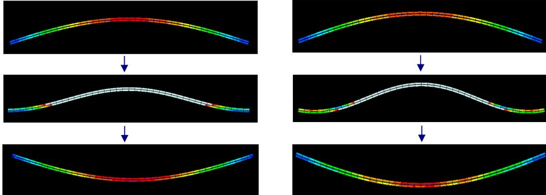
Figure 7: Snap-through of three-layer arch caused by induced deformation of the layers:
