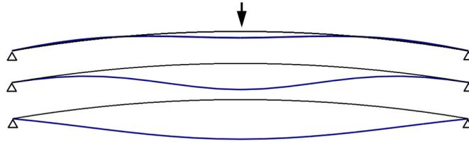
Figure 5: Snap-through of arch caused by point load: a) state just before snap-through, b) snap-through, c) state just after snap-through
