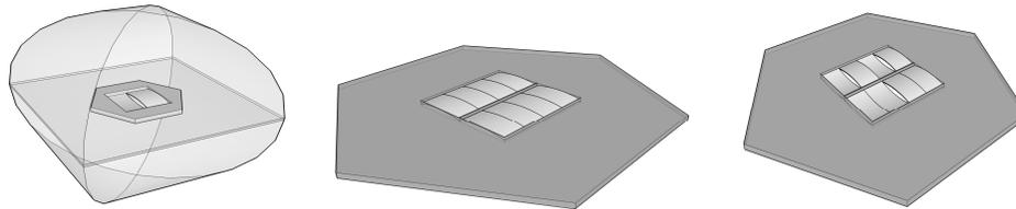
Figure 4: General view: absorber equipped with bistable valve, the valve composed of a matrix of bistable shell elements
