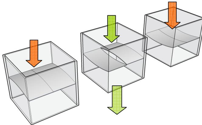
Figure 3: Simple bi-stable valve: initial closed state, intermediate open state, final closed state
