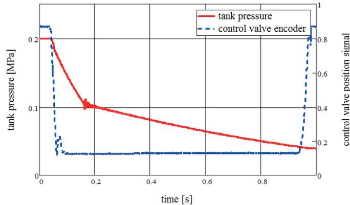
Figure 12: Test results: tank pressure and control valve position signals
