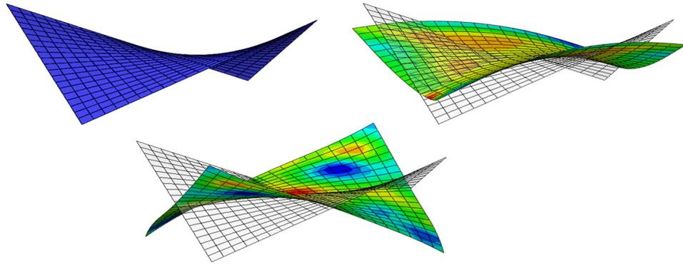
Figure 8: Snap-through of hyperbolic paraboloid (rectilinear surface) caused by points loads applied at corners: a) initial configuration, b) intermediate stage of the process, c) final configuration
