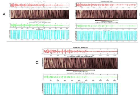
Fig. 3. Signal envelope decomposition from 3 phantoms
