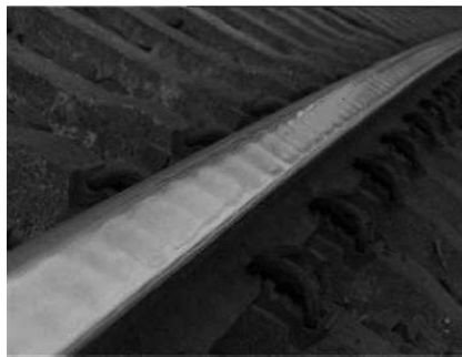
Fig. 1. Typical rail corrugation due to bad rolling conditions [Photo R. Konowrocki]
