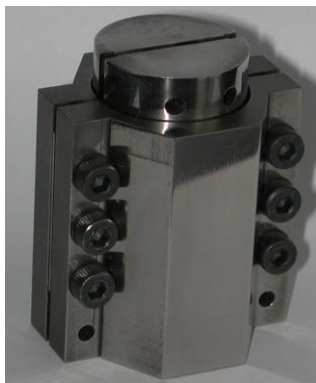
Fig. 4. The shear device for investigations at high strain rates as well as in quasi-static conditions.
