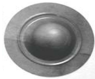
Fig. 2: The experimentally deformed shape of sheet metal
