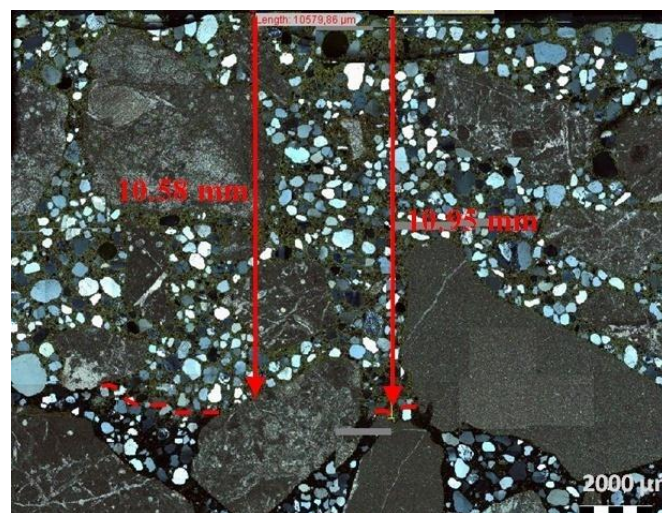
Figure 7. Thin-section view of concrete with limestone aggregate and CEM II/B-M (V-W) with visible carbonation front, after 56 days of exposition in 1% CO 2 , XPL, scale bar = 2000 μm.
