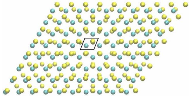
Figure 1: The structure of the two dimensional sheet of Single-Layer MoS<sub>2</sub>
