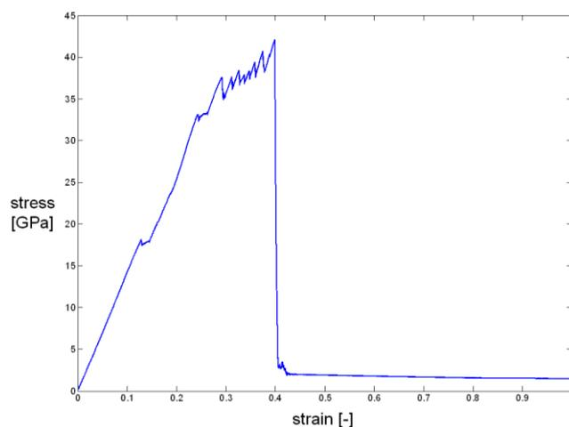
Figure 2: The results of tensile test for SLMoS<sub>2</sub>
