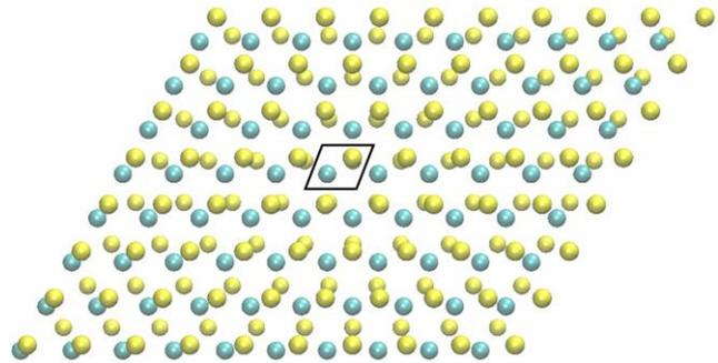
Figure 1: The structure of the two dimensional sheet of Single-Layer MoS<sub>2</sub>
