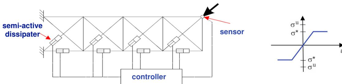
Fig. 2. Adaptive structure equipped with fluid-based semi-active dissipaters [9]: a) general scheme, b) exemplary characteristics of the dissipater
