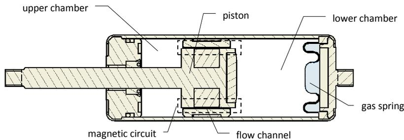
Fig. 1. Magneto-rheological damper: a typical example of fluid-based semi-active dissipater [4]
