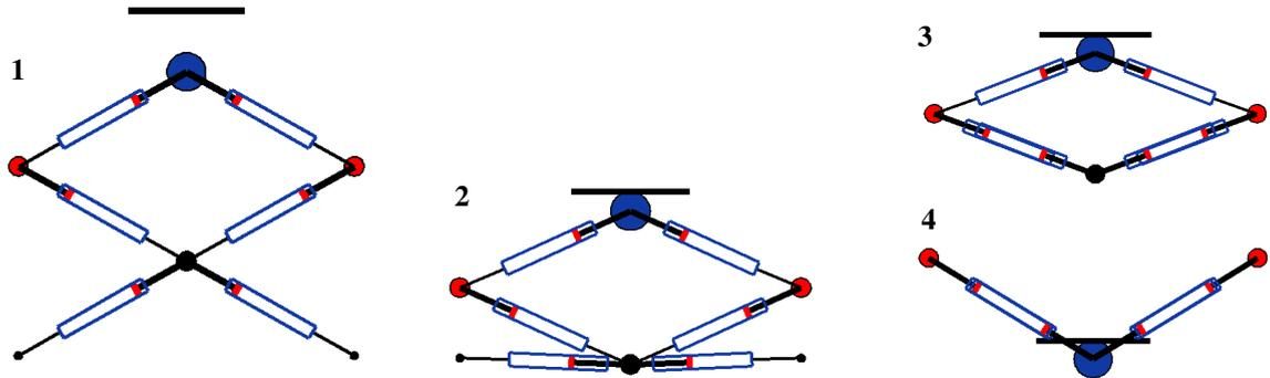
Fig. 3. Various folding sequences of adaptive multifolding skeletal structure
