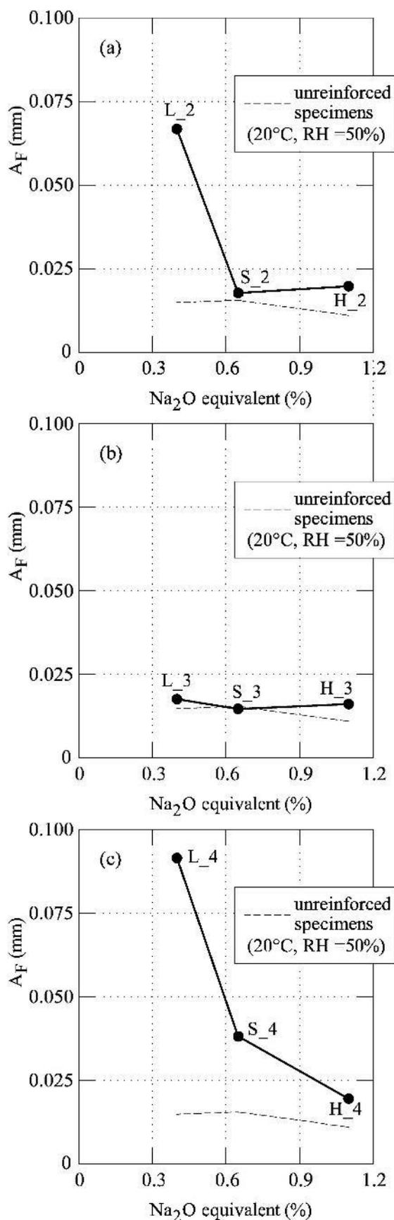
Fig. 7: The area  $A_F$  measured in the three point bending tests: (a) specimens cured for 27 days in normal conditions (20°C, RH = 50%); (b) specimens cured for 27 days in water (20°C); (c) specimens cured for 3 days in water (20°C).
