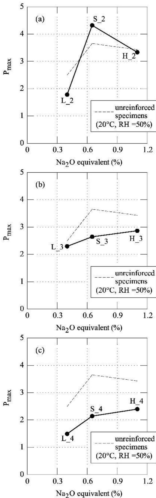
Fig. 5: The flexural strength  $P_{max}$  measured in the three point bending tests: (a) specimens cured for 27 days in normal conditions (20°C, RH = 50%); (b) specimens cured for 27 days in water (20°C); (c) specimens cured for 3 days in water (20°C).
