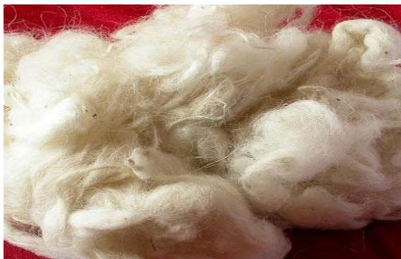
Fig. 1: Sheep wool used to reinforce mortars.
