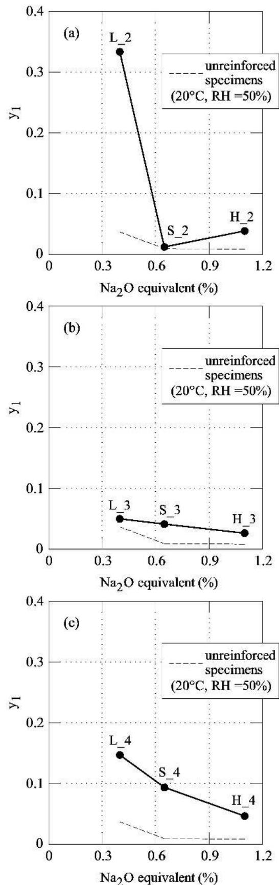
Fig. 6: The residual stress  $y_1$  measured in the three point bending tests: (a) specimens cured for 27 days in normal conditions (20°C, RH = 50%); (b) specimens cured for 27 days in water (20°C); (c) specimens cured for 3 days in water (20°C).
