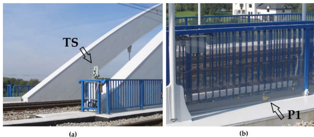
Figure 6. View of the trigonometric survey: (a) Total Station TS location; (b) prism P1 location.
