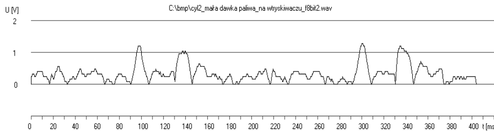
Fig. 8. Acoustic signal registered on the stub inlet to the injector in the situation when the fuel pump was out of trim and supplies the injector with insufficient fuel volume. The signal amplitude is smaller than that shown in Fig. 4.
