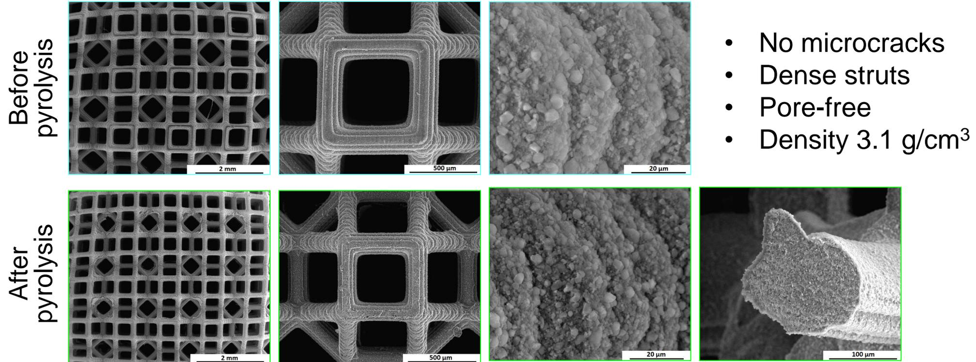
Some unreacted  $\text{Al}_2\text{O}_3$  particles at the struts' surface
