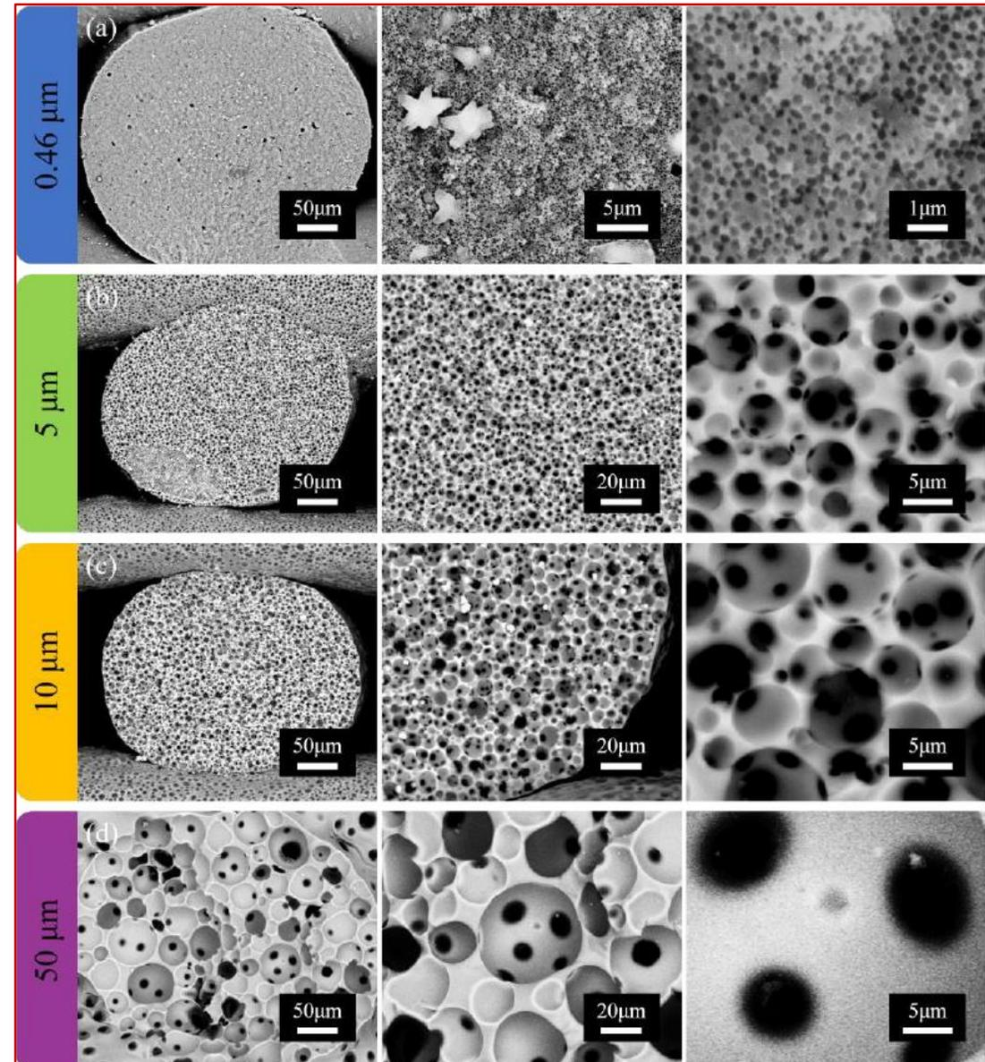
Different filler size (80 vol% PMMA filler)
