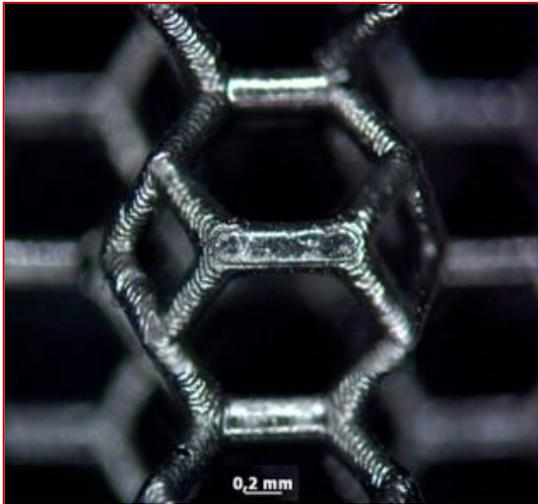
→ Control of the final dimensions of the printed ceramic part
