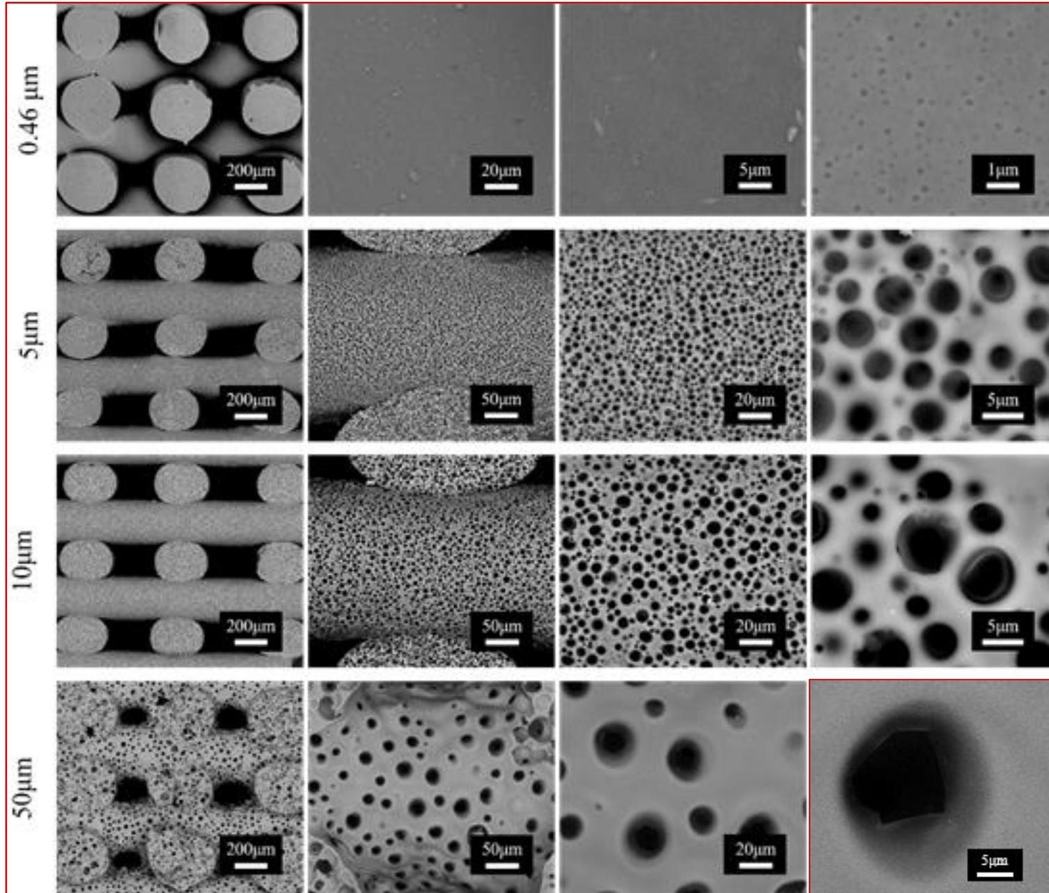
Surface of filaments from scaffolds fabricated using inks containing 80 vol% of particles of different size: 5, 10, 50  $\mu\text{m}$  (left image: cross-section of the scaffolds)
