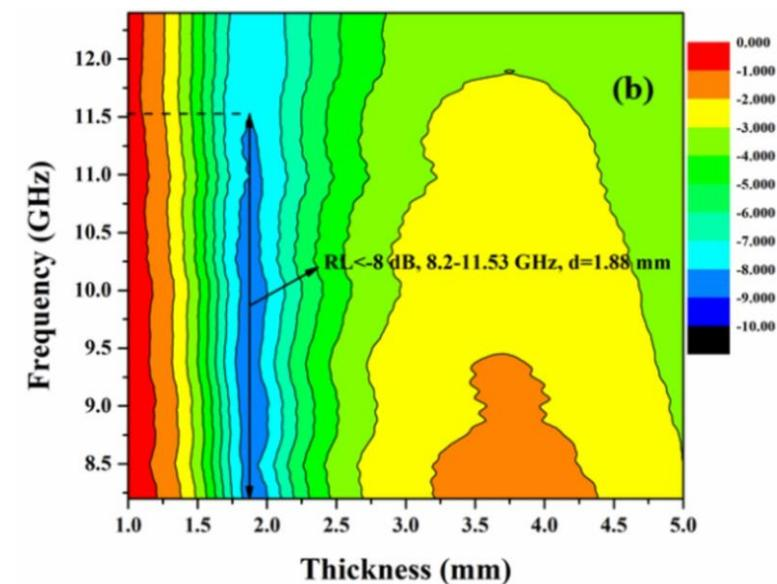
EMW absorption of SiOC ceramics with integration of structure and function
