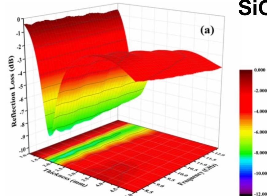
Reflection Loss of 3D-SiOC ceramics in X band
