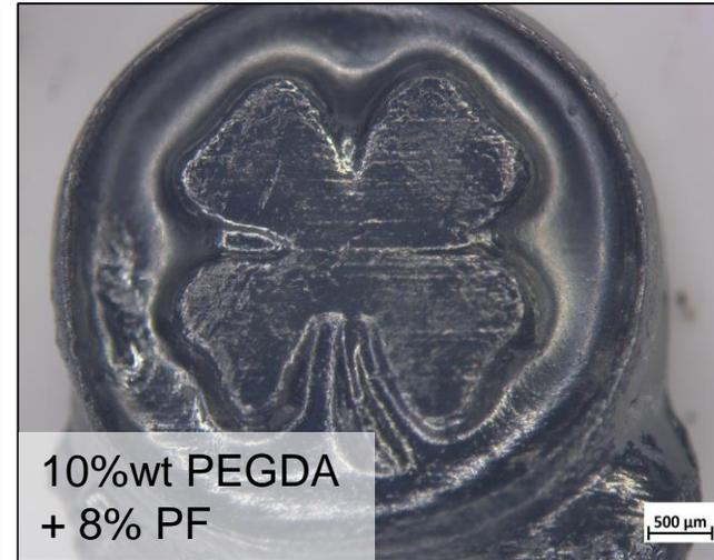
+ crack-free components
