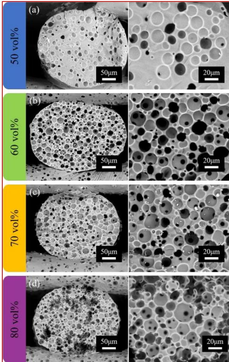
Different vol% PMMA filler (25  $\mu\text{m}$ )
