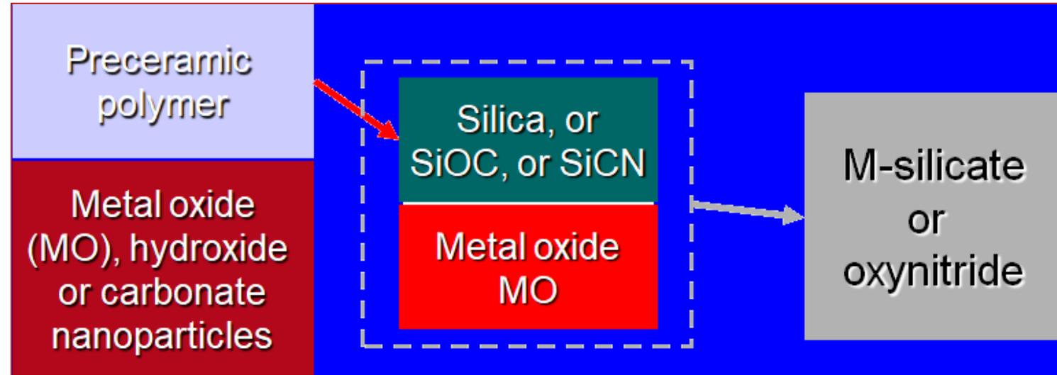
Several bioceramic (silicate) phases can be obtained
