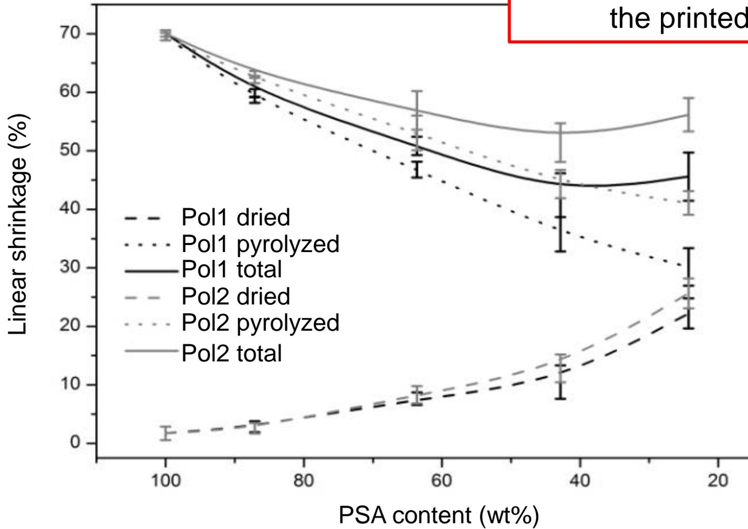
Average drying shrinkage, pyrolysis shrinkage and total shrinkage of blends
