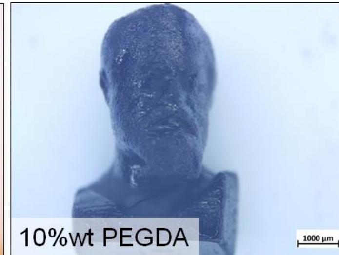
**Cracks** upon pyrolysis → hindered release of decomposition gases → partial substitution of UDMA with **PEGDA** + addition of a **low T release** component (PF):
