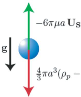
A free-body diagram of a blue sphere. A green arrow points upwards labeled  $-6\pi\mu a U_S$ . A red arrow points downwards labeled  $\frac{4}{3}\pi a^3(\rho_p - \rho_f) g$ . A black arrow points downwards labeled  $g$ . A red arrow points downwards labeled "Stokes' velocity".
