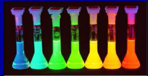
Fluorescence of CdSe quantum dots D. Talapin, University Hamburg
