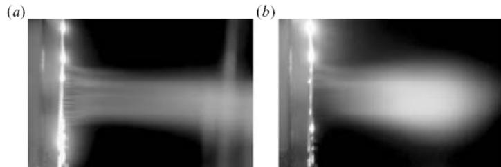
Ethanol spray as issued from device D55 for  $Q = 50 \text{ ml h}^{-1}$ ,  $\Delta P = 530 \text{ mbar}$ , with: (a) 0 V, (b) 1130 V.
