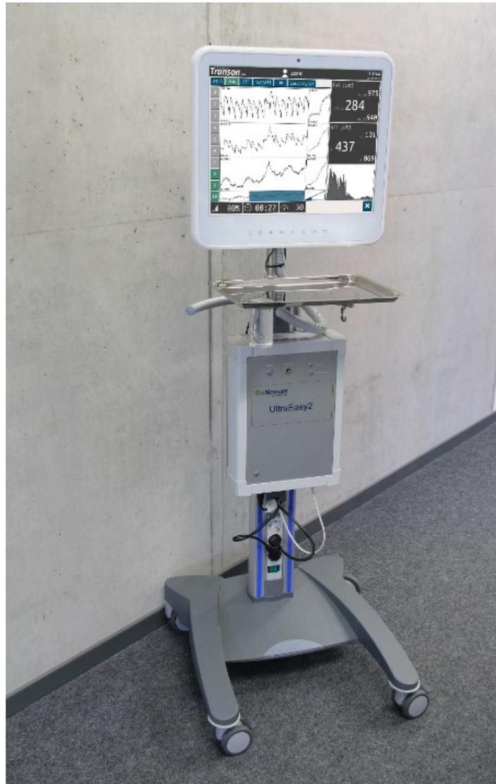
Figure 62: Shows the ACG System- UltraEASY 2 used for clinical trials. It consists two ACG probes joined by a strap on the patient's head connected to an output device with touchscreen to record and data presentation. All components are assembled to a trolley to be transportable
