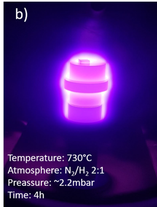
Fig. 1—Nitriding of HEA; (a) CALPHAD (ThermoCalc) predictions of the stable phases; (b) sample during nitriding.
