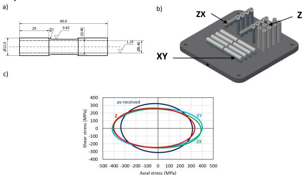
Thin-walled tubular specimen for yield surface determination (a); printing orientation of specimens on the build plate (b); comparison of the yield surfaces for three printing orientations and the same material in the as-received state for 0.005% plastic offset strain (c)
