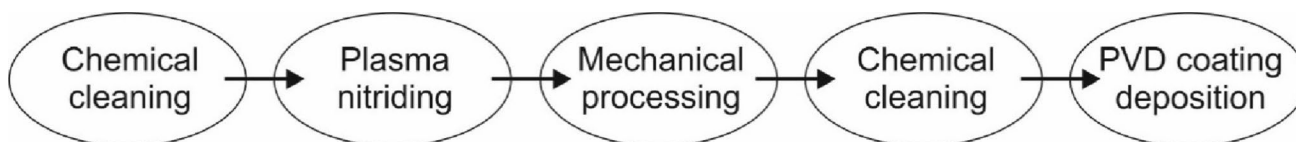
Fig. 1 Schematic of the hybrid surface treatment applied to the investigated forging dies
