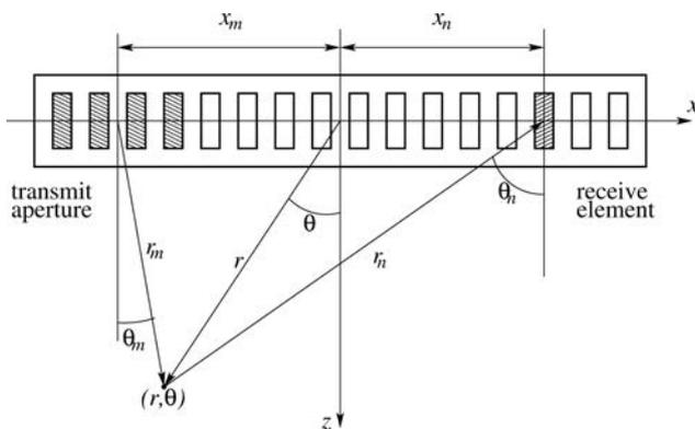
Fig. 1. The transmit and receive elements combination and the focus point in the MSTA method.
