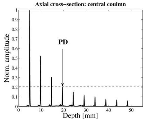
Fig. 3. Evaluation of the penetration depth: PD is the location of deepest reflector for which the normalized amplitude exceeds the given level in the axial cross-section coinciding with the central column of point reflectors.
