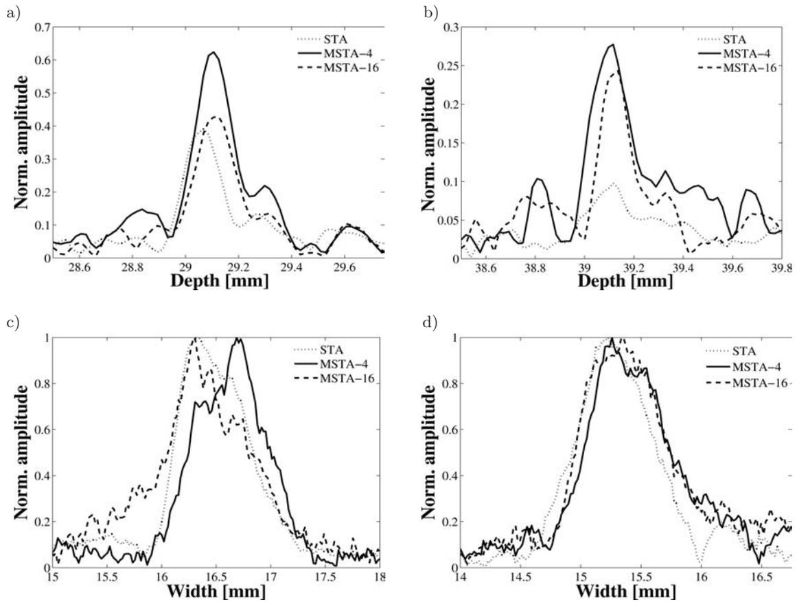
Fig. 8. a), b) Axial cross-sections of the phantom line #1885 at different depths and c), d) lateral cross-sections at depths 10 mm and 60 mm of the reflectors situated on the right hand side of the phantom. The transmit apertures with  $N_t = 1, 4, 16$  are compared.
