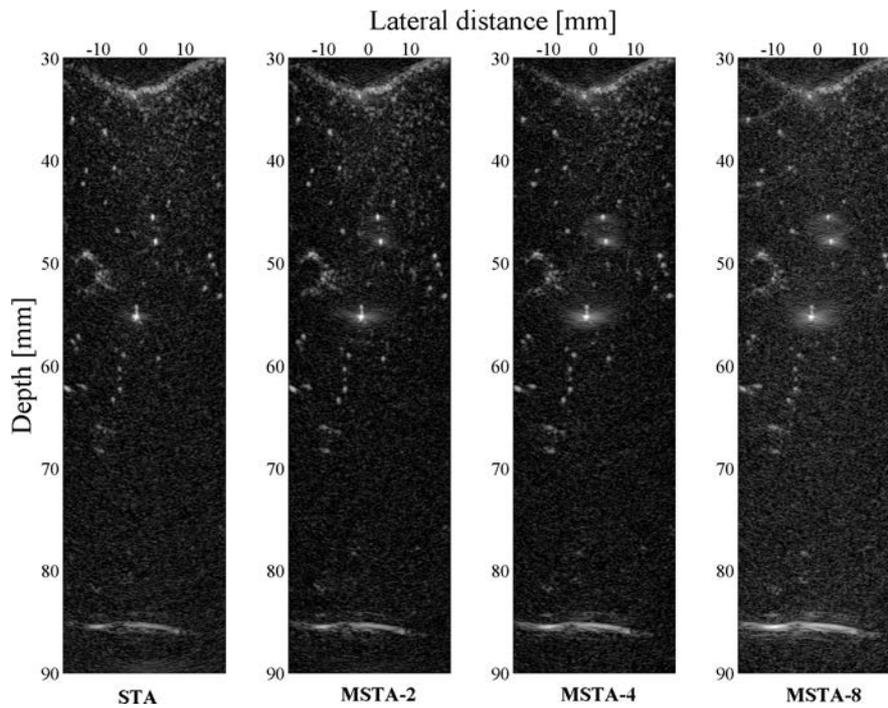
Fig. 9. 2D visualization of beef liver pattern study *in vitro* for different transmit aperture sizes: a single-element aperture – STA and 2,4,8-element aperture (MSTA). All images are displayed over the 40 dB dynamic range.
