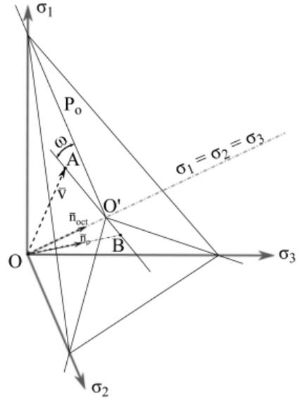
Fig. A4. Geometrical interpretation of the vector  $\mathbf{n}_p$  normal to the characteristic plane and its relation to the stress vector  $\mathbf{v}$  in the principal stress space
