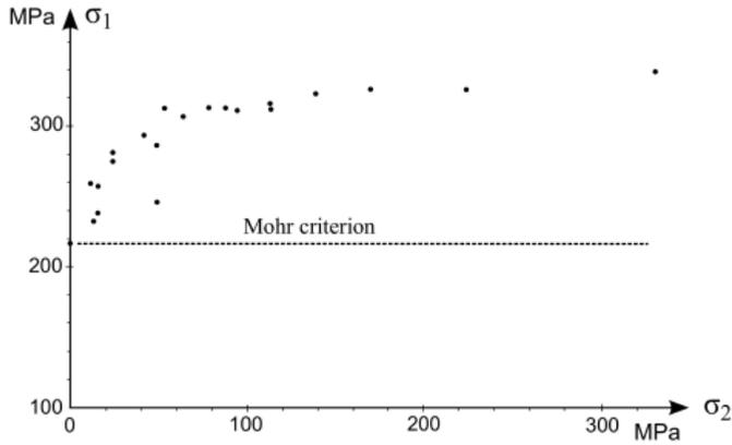
Fig. 5. Effect of the intermediate principal stress  $\sigma_2$  on the strength of Dunham Dolomite (Mogi, 1967)
