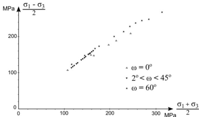
Fig. 4. The relation between shear stress  $\tau_{\max} = (\sigma_1 - \sigma_3)$  and normal stress  $\sigma_n = (\sigma_1 + \sigma_3)$  for Dunham Dolomite – results of tests from (Mogi, 1967)
