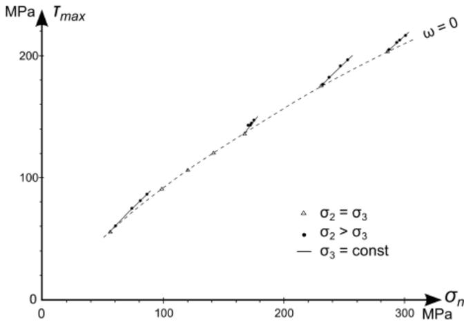
Fig. 1. The relation between shear stress  $\tau_{max} = \frac{1}{2}(\sigma_1 - \sigma_3)$  and normal stress  $\sigma_n = \frac{1}{2}(\sigma_1 + \sigma_3)$  in Sandstone – results of tests from (Akai & Mori, 1970)
