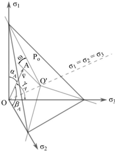
Fig. A1. Geometrical interpretation of the state of stress in the principal stress space – plane  $P_o$  is the octahedral one
