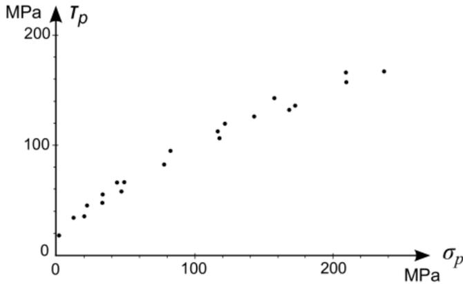
Fig. 3. The relation between shear  $\tau_p$  and normal  $\sigma_p$  stresses acting on characteristic planes in Sandstone for  $P = 0,35$  – results of tests from (Akai & Mori, 1970)
