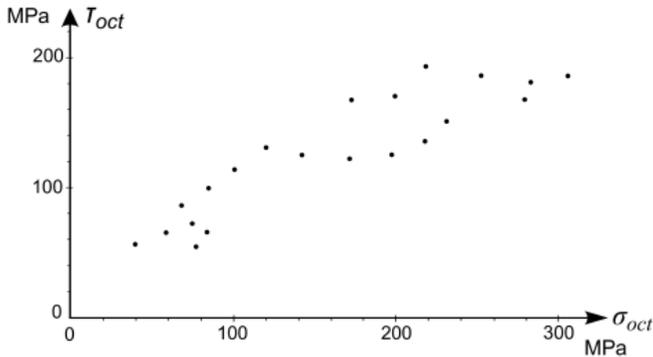
Fig. 2. Failure stress  $\tau_{oct}$  as a function of the mean stress  $\sigma_{oct}$  for Sandstone – results of tests from (Akai & Mori, 1970)
