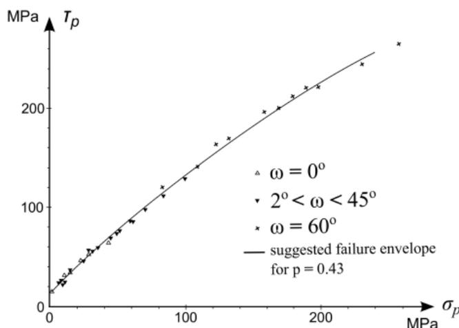
Fig. 7. The relation between shear  $\tau_p$  and normal  $\sigma_p$  stresses acting on characteristic planes in Dunham Dolomite for  $P = 0,43$  – results of tests from (Mogi, 1967)
