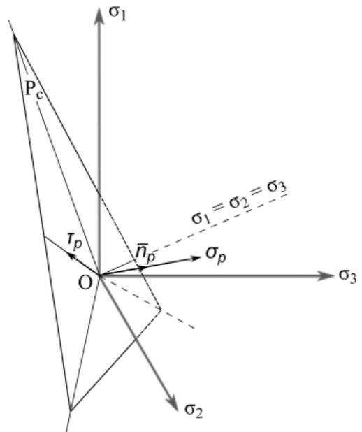
Fig. A2. Characteristic plane  $P_c$  with the stresses  $\tau_p$ ,  $\sigma_p$  and normal  $\mathbf{n}_p$
