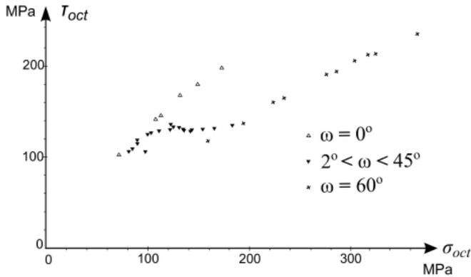
Fig. 6. Failure stress  $\tau_{oct}$  as a function of the mean stress  $\sigma_{oct}$  for Dunham Dolomite – results of tests from (Mogi, 1967)
