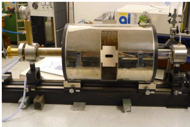
Fig.1 Reactor for synthesis of carbon nanotubes. In the centre of the furnace - inspection window. On the left side of the furnace the brass collector and the mechanism for target rotation.
