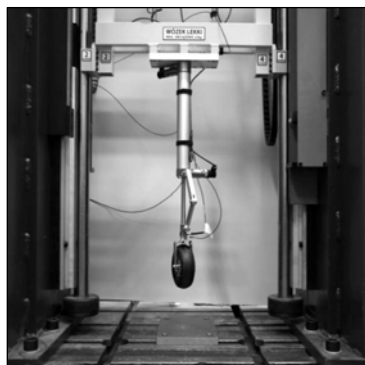
Figure 7 Drop-test stand with adaptive absorber
