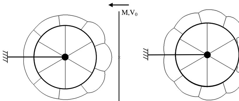
Figure 4 - Two dimensional model of collision: initial state and resulting deformation.
