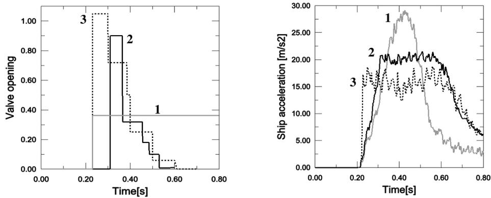
Figure 7 - Comparison of three control strategies involving pressure release: a) applied valve opening, b) resulting ship acceleration.
