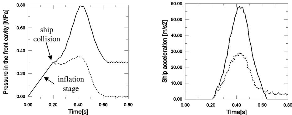
Figure 5 - Semi-active acceleration mitigation without (continuous line) and with pressure release (dashed line): a) overpressure in the front chamber, b) corresponding ship acceleration.
