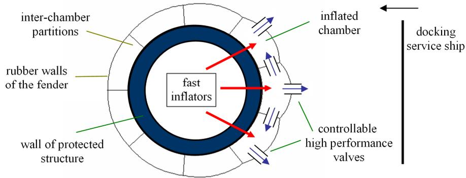
Figure 2 - Horizontal projection of the pneumatic fender protecting the tower.
