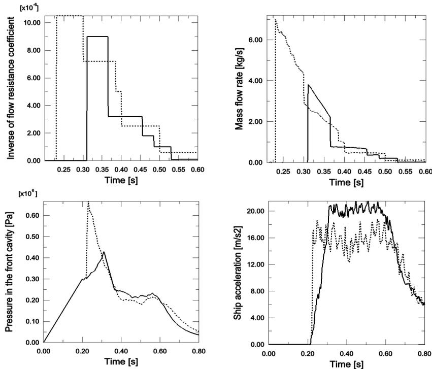
Figure 6 - Two strategies of active acceleration mitigation: i) pressure only released during impact (continuous line), ii) additional inflation at the beginning of impact (dashed line).
