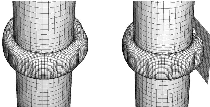
Figure 3 - Three dimensional model: a) initial fender inflation, b) deformation during ship impact
