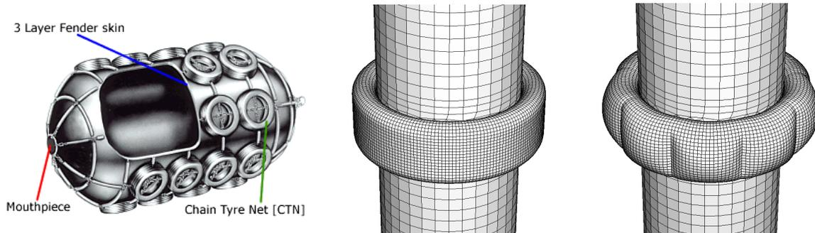
Figure 1 - Pneumatic fenders: a) standard passive Yokohama-type fender, b) deflated torus-shaped fender, c) torus-shaped fender with uniform inflation of all chambers.
