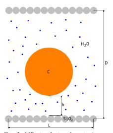
Fig. 2: MD simulation domain (not to scale) with one 24nm colloidal carbon particle suspended in water between two quartz walls. L=D=310.5nm.
