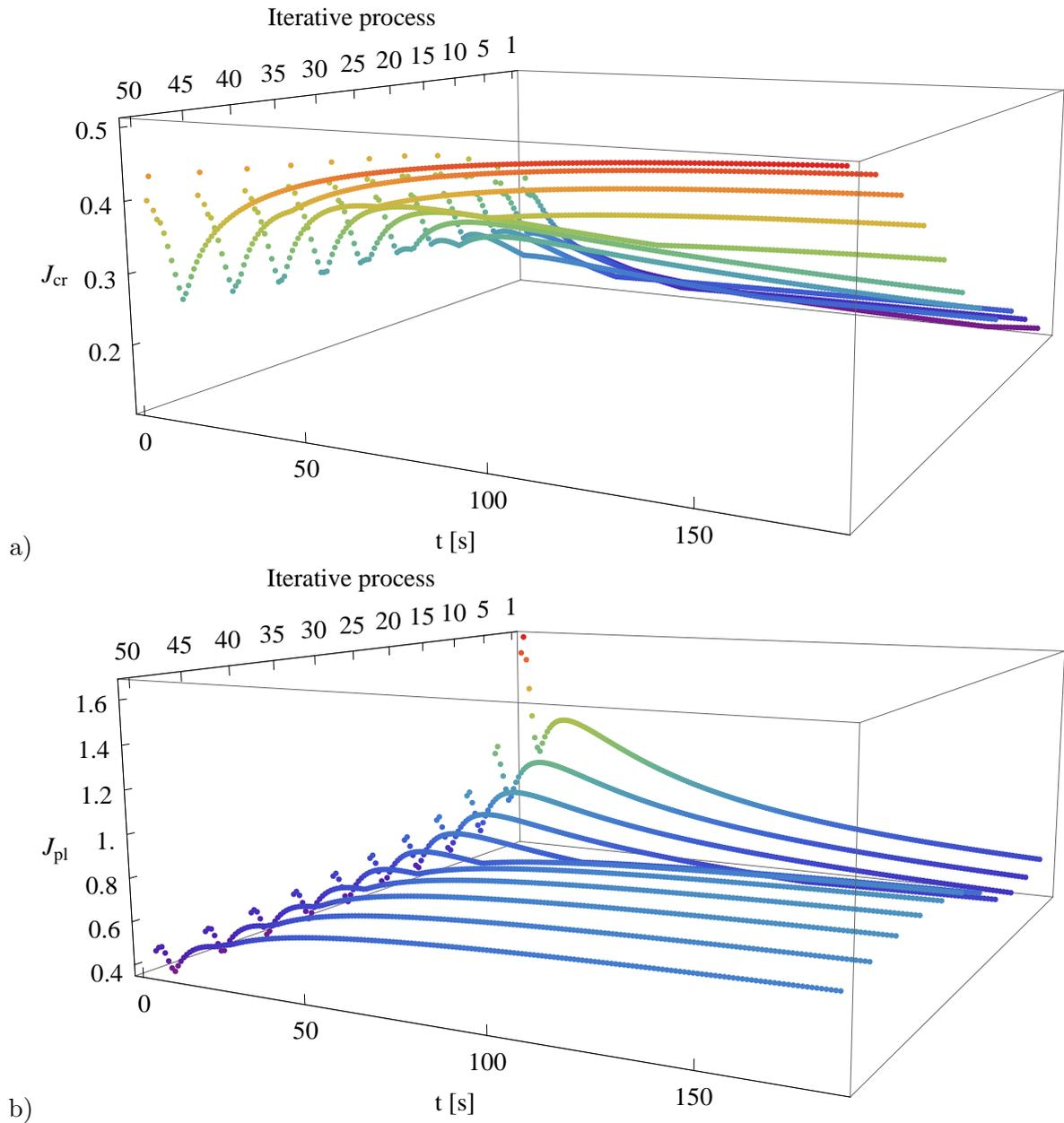
Figure 3: Iterative process of rebuilding ceramic volume fraction; a) and b) show evolution of crack strength parameter  $J_{cr}$  and yield strength parameter  $J_{pl}$  respectively, see Eqs. (7) and (6). Thermomechanical loading (combustion process) starts at  $t = 0$ . There are 50 transient thermo-mechanical processes, each one for different ceramic phase distribution.
