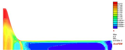
Figure 4: Ceramic exhaust valve analysis with optimal (for  $\beta = 1.0$  in Eq. (1)), inhomogeneous distribution of ceramic phase.
