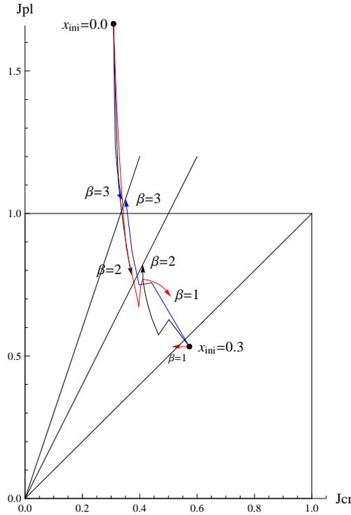
Figure 5: Paths of optimization processes with the parameter  $\beta$  in Eq. (1) equals one, two, and three. Optimizations start from the state of homogeneous density of ceramic phase equal to  $x_{ini} = 0.0$  or  $x_{ini} = 0.3$ .
