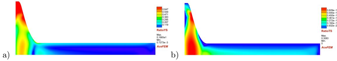
Figure 2: Analysis of ceramic exhaust valve with initial, homogeneous distribution of ceramic phase  $Al_2O_3$  within  $NiAl$  matrix ( $x_{ini} = 0.0$ ); a) and b) distribution of yield strength and crack strength parameters  $J_{pl}$  and  $J_{cr}$ , defined by Eqs (6) and (7) respectively at time  $t = 2$  s of the process.
