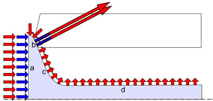
Figure 1: The schematic representation of the axisymmetric valve model used in the finite element simulations. The valve is subjected to mechanical loading at interfaces a (pressure) and b (contact with the engine), while thermal fluxes act at interfaces a, b, c, and d (marked with red colour).
