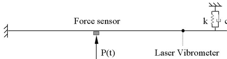
Figure 1. Experimental test stand: damaged structure
