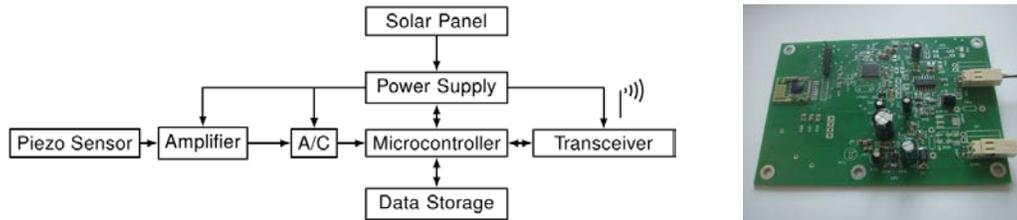
Figure 8. Wireless sensor: block diagram and PCB implementation.
