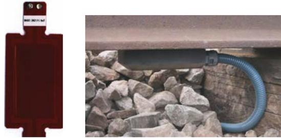
Figure 4. WIM piezoelectric PFC sensor.
