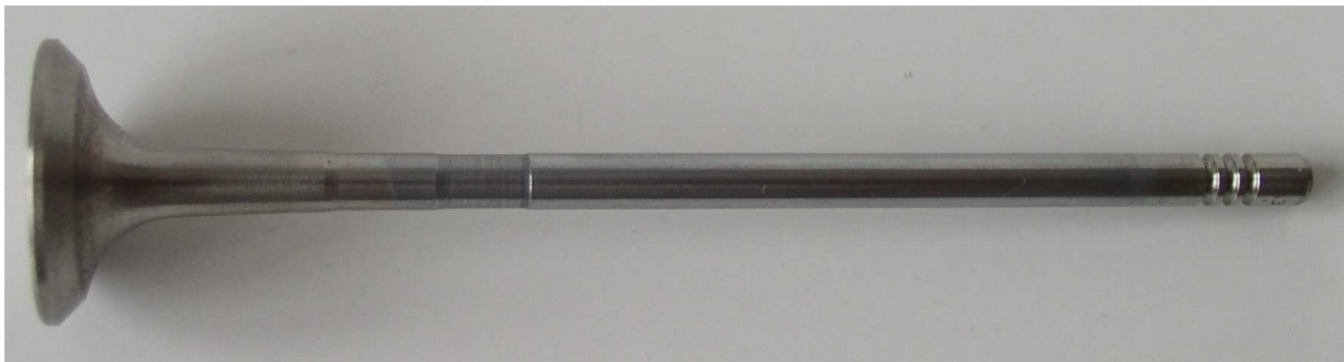
Fig. 1. An example of light valve of a graded metal matrix composite under investigation (courtesy of Institute of Materials Research of Slovak Academy of Sciences, Bratislava).
