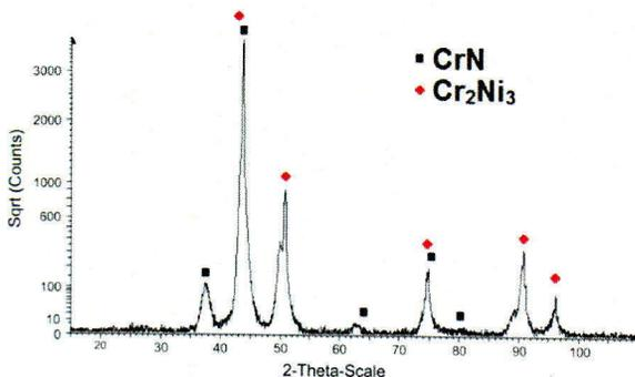
Fig. 2 X-ray diffraction pattern of the layer formed on an Inconel 740.
