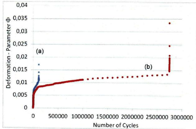
Fig. 4 Changes of the deformation parameter versus number of cycles to failure in the Inconel 740 nickel alloy: (a) as-received, (b) with a CrN+Cr<sub>2</sub>Ni<sub>3</sub> layer and stress amplitude of 500 MPa.
