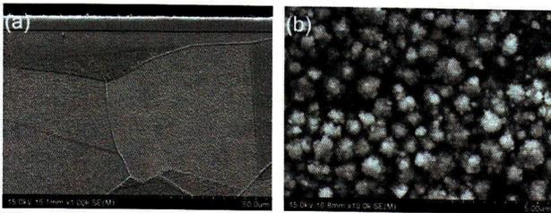
Fig. 1 Cross-section, (a), and surface, (b), morphology of the CrN+Cr<sub>2</sub>Ni<sub>3</sub> layer produced on Inconel 740 nickel alloy.
