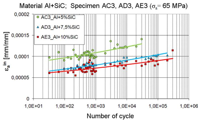
**Figure 6.** Inelastic strain amplitude  $\epsilon_a^{in}$  for selected cycles
