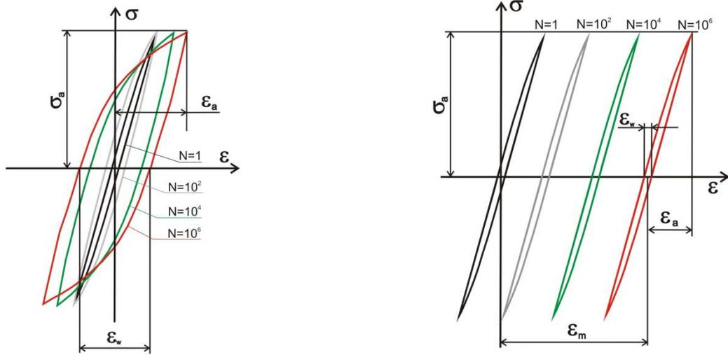
**Figure 2.** Hysteresis loops depending on the damage mechanism: (a) cyclic plasticity, (b) ratcheting
