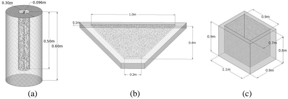
Figure 1.1 Measurement molds (a) 1D (b) 2D (c) 3D.
