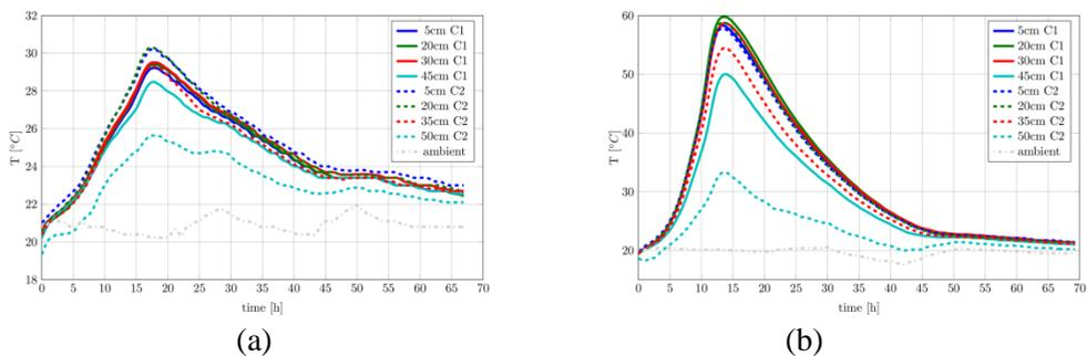
Figure 3.1 Temperature evolution during hardening of concrete in 1D molds (a) mixture A and (b) mixture B. Solid lines denote measurement in configuration C1, and dashed lines in configuration C2. Sensor positions in each configuration are listed in the legend.
