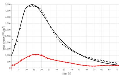
Figure 3.2 Heat source determined by means of inverse heat transfer problem solution for mixture A (red points) and mixture B (black points). Solid lines denote fitted analytical approximations of these functions.
