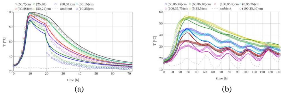
Figure 3.4 Model validation: (a) 2D case – mixture B (b) 3D case (cross section) mixture A. Lines denote numerical solution, circles denote measurements.
