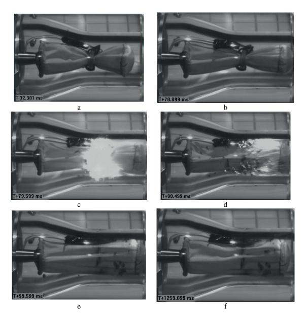
Figure 11: The HPV sequence of operation (beginning from left hand side)
