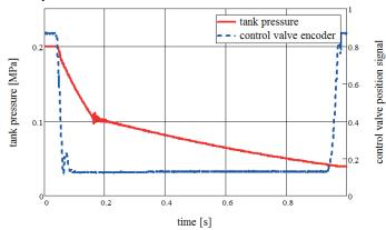
Figure 12: Test results: tank pressure and control valve position signals
