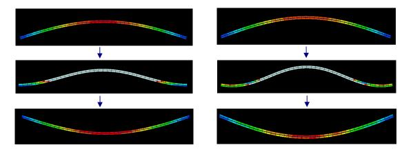
Figure 7: Snap-through of three-layer arch caused by induced deformation of the layers: a) shortening of the top layer, b) elongation of the bottom layer
