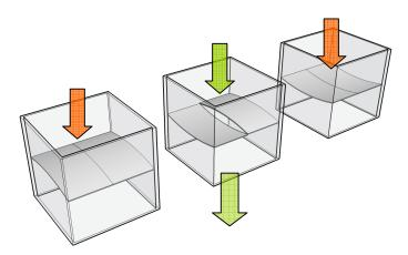
Figure 3: Simple bi-stable valve: initial closed state, intermediate open state, final closed state
