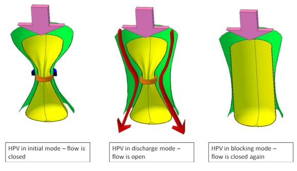
Figure 10: The HPV sequence of operation (beginning from left hand side)
