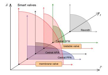
Figure 2: Comparison of valves' characteristics (P-blocking force, t-reaction time, δ-stroke).
