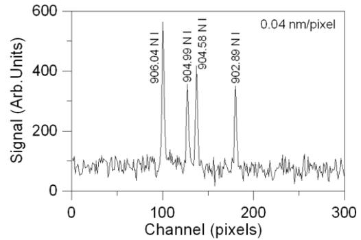
Fig. 3. Spectral lines of atomic nitrogen in infrared region
