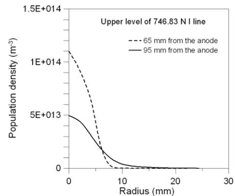
Fig.4. Population density of upper level of 746.83 nm N I line
