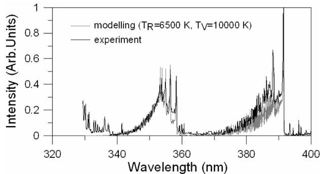
Fig. 6. Experimental and synthetic spectra of molecular bands at a distance 95 mm from the anode
