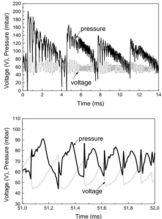
Fig.2. Arc voltage and pressure recorded during 14 and 1 ms at arc current 245 A and nitrogen flow rate 0.8 g/s introduced into arc and 0.6 g/s into plasma jet
