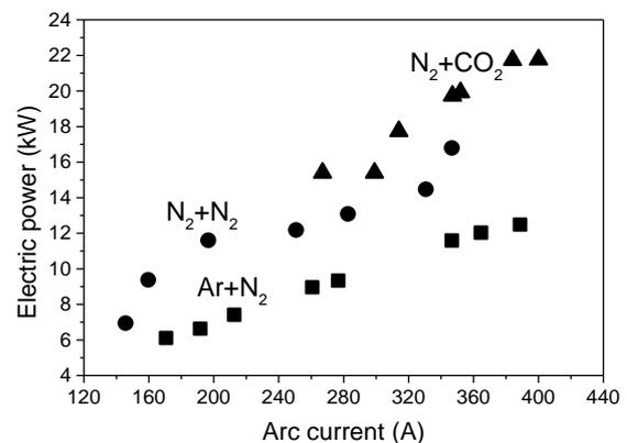
Fig.1. Input electric power for gas flow rate 0.8g/s injected into arc and 0.6g/s into plasma jet at pressure 6kPa; ■ - argon arc and nitrogen introduce into plasma jet; ● - nitrogen arc and ● - nitrogen or ▲ - carbon dioxide introduce into plasma jet
