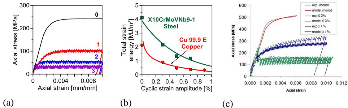
Fig. 2. Comparison of tensile characteristic (0) of the copper with stress-strain curves obtained during monotonic tension assisted by the torsion-reverse-torsion cycles for strain amplitude equal to:  $\pm 0.3\%$  (1),  $\pm 0.5\%$  (2),  $\pm 0.7\%$  (3) - (a), total strain energy versus cyclic strain amplitude (b), comparison of experimental and numerical results (c).
