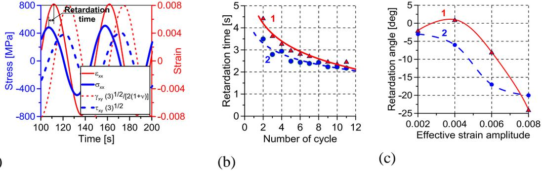
Fig. 1. The results for the 2024 alloy tested under cyclic loading along the circular strain path: (a) stress and strain signal components versus time at the cyclic strain amplitude equal to  $\pm 0.8\%$ ; (b) retardation time as a function of cycle number; (c) retardation angle versus effective strain amplitude; 1 and 2 - axial and shear components, respectively
