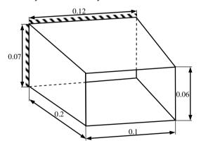
Figure 1: Box beam – dimensions and bearing
