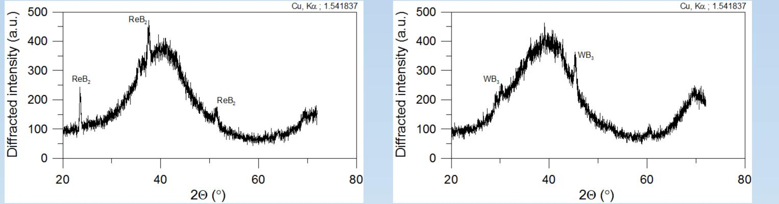
ReBN and WBN coatings are amorphous. XRD diffractogram contain only a single peaks from the crystalline phase.
