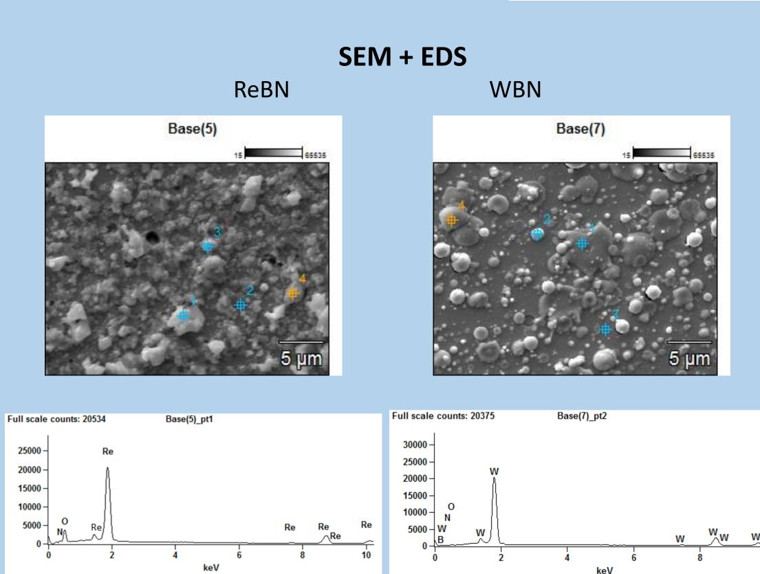
ReBN and WBN layers were characterized by low nitrogen content. The ReBN layers have low density and irregular structures on the layers surface. The WBN layers are dense but are composed mainly by droplets.
