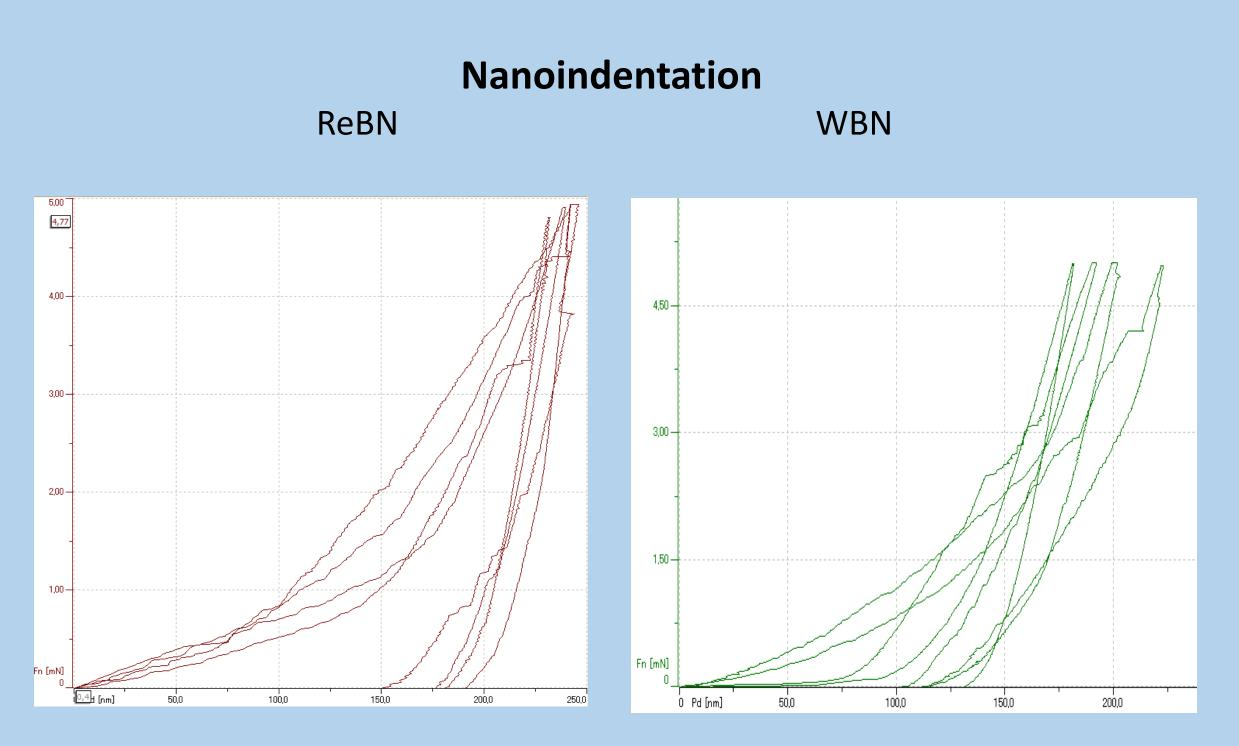
Results of Vickers hardness of ReBN sample (a) 5685.6 MPa and WBN sample (b) 9004.3 MPa,
