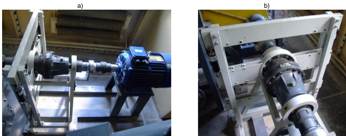
Figure 1: Coal pulverizer drive system (a) and the damper with the linear MRF actuators (b)
