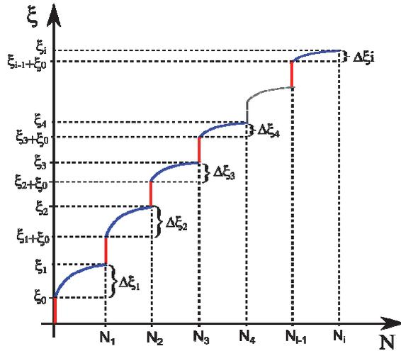
Figure 2: The mechanism of damage evolution
