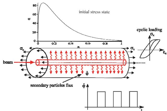
Figure 1: Coaxial target – detector configuration
