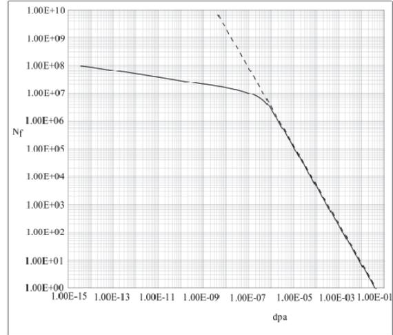
Figure 3: Number of cycles to failure  $N_f$  as a function of  $dpa$
