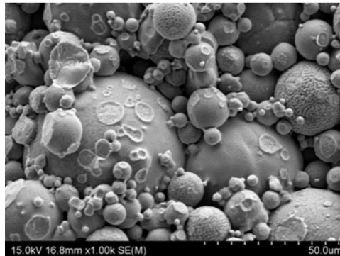
Fig. 1. Microstructure of NiAl at an early stage of sintering.
