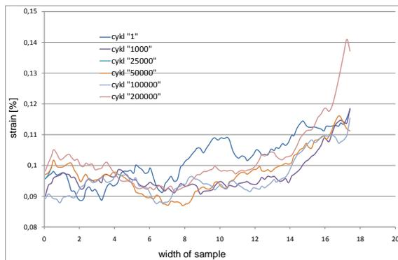
**Fig. 3** Lateral profiles of strain changes in the cross-section with the maximum values.
