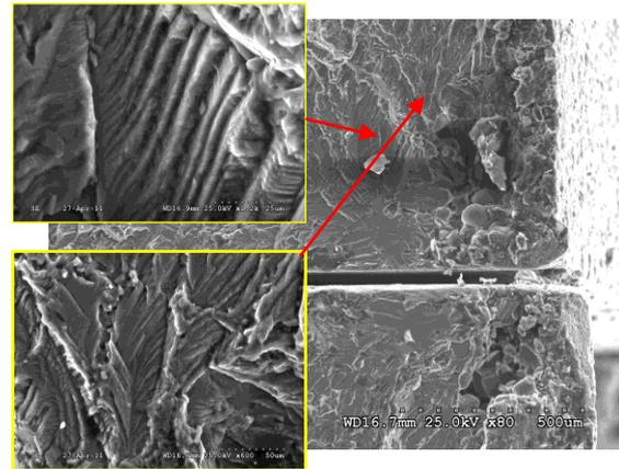
**Fig. 4** Sample fracture with the pore visible on both parts and the close-up of fatigue fringes in its vicinity
