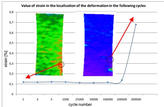
**Fig. 2** Distortion location and its development in consecutive cycles
