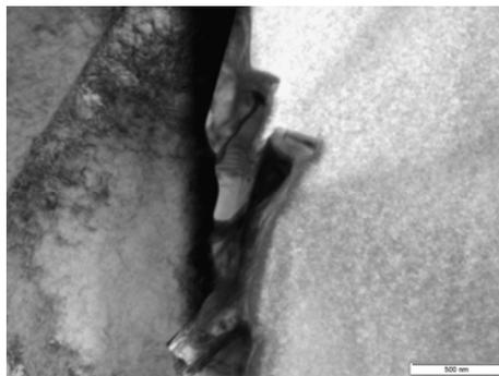
**Fig. 5.** TEM image of alumina-copper grain boundary.
