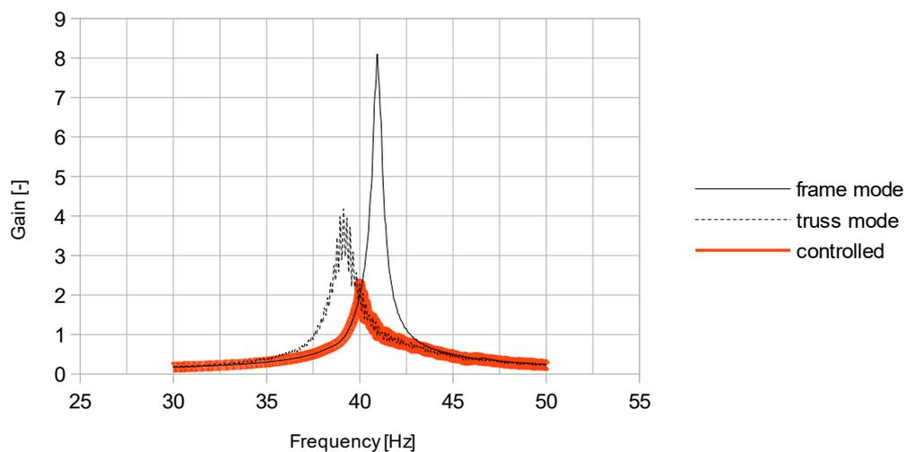
**Figure 7:** Frequency response of the controlled frame for 2<sup>nd</sup> eigen mode (measurement point P16).
