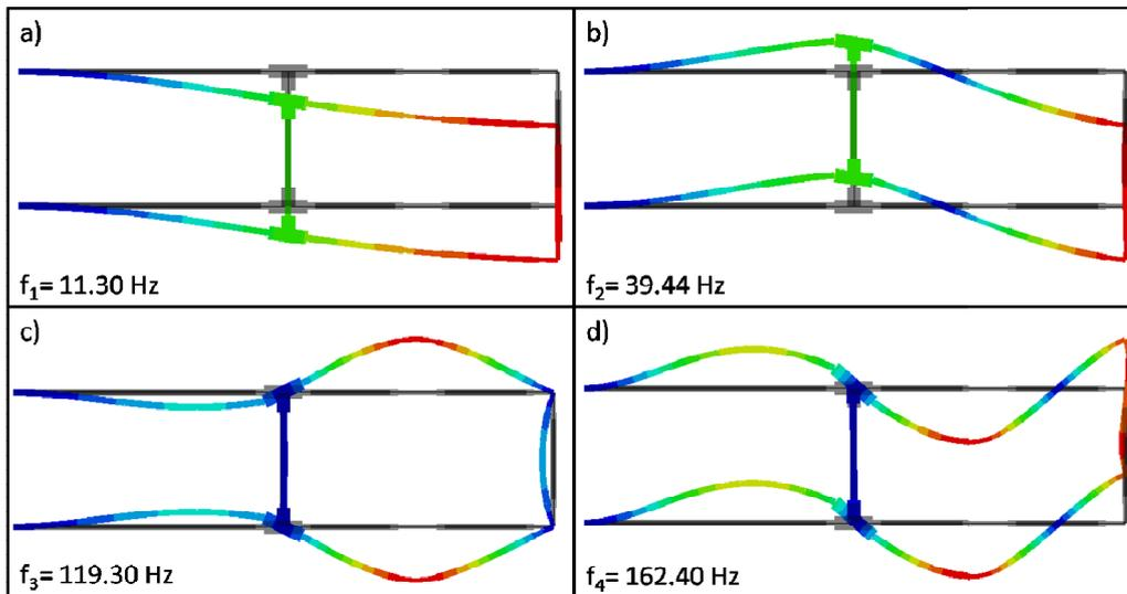
**Figure 2:** First four mode shapes of numerical model.
