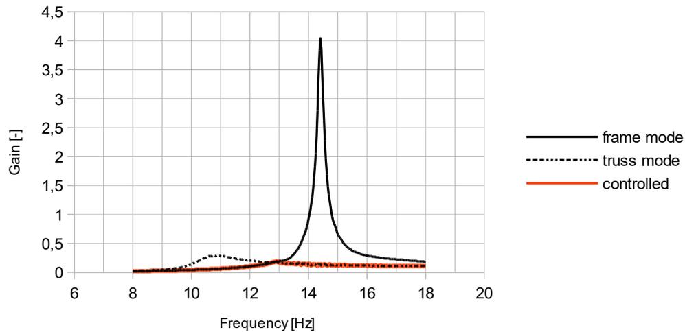
**Figure 6:** Frequency response of the controlled frame for the 1<sup>st</sup> eigen mode (measurement point P16).
