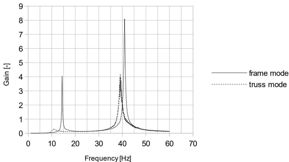
**Figure 5:** Frequency response of the frame for the 1<sup>st</sup> and 2<sup>nd</sup> eigen mode (measurement point P16).
