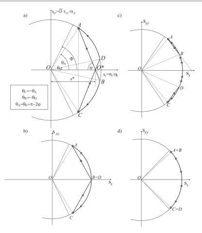
FIG. 5. Steady state cycles representation in the  $s_x$ ,  $s_{xy}$ -plane a) the case  $\eta > \eta_m(\gamma_m)$ , b) the case  $\eta = \eta_m(\gamma_m)$ , c) the case  $\eta_l(\gamma_m) < \eta < \eta_m(\gamma_m)$ , d) the case  $\eta > \eta_l(\gamma_m)$ .
