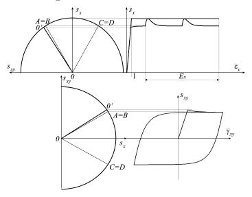
FIG. 9. Variation of the tensile stress path and the hysteresis loop of shear stress-strain response in the course of cyclic deformation,  $\eta < \eta_l$  regime  $\mathcal{A}$ : no elastic unloading.
