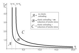
FIG. 7. The regimes  $\mathcal{A}, \mathcal{B}, \mathcal{C}$  of cyclic response in the plane of process parameters  $\eta$ ,  $\gamma_m \ (m = m_{Al} = 0.128).$
