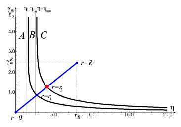
FIG. 24. Three different stress regimes within a cylinder subjected to monotonic extension and cyclic torsion.
