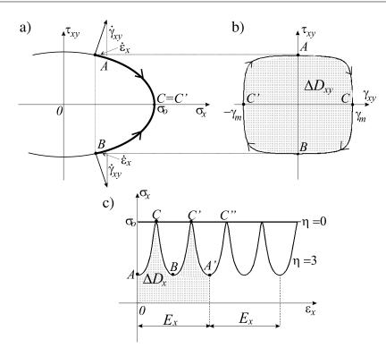
FIG. 3. Harmonic shear strain control: a) stress path, b) shear stress-strain hysteresis loop, c) axial stress variation.
