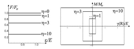
FIG. 20. The cross-sectional force and moment variation in the steady cyclic state.
