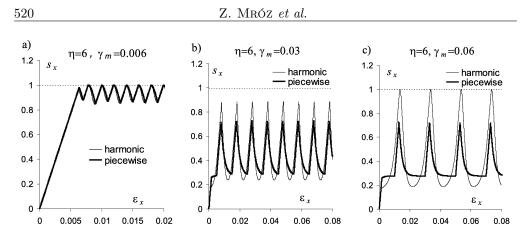
FIG. 17. Comparison of the tensile stress paths for piecewise linear and harmonic shear strain controls (E = 77000 MPa,  $\nu = 0.4$ ,  $\sigma_0 = 500$  MPa,  $\eta = 6$ ), a)  $\gamma_{m1} = 0.006$ , b)  $\gamma_{m3} = 0.03$ , c)  $\gamma_{m2} = 0.06$ . Relative parameter values:  $\varepsilon_0 = \sigma_0/E \sim 0.0065$ ,  $\gamma_m/\varepsilon_0 = 0.924$ ; 4.62; 9.24.
