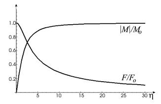
FIG. 21. Variation of axial force and twisting moment with the parameter  $\eta$ .
