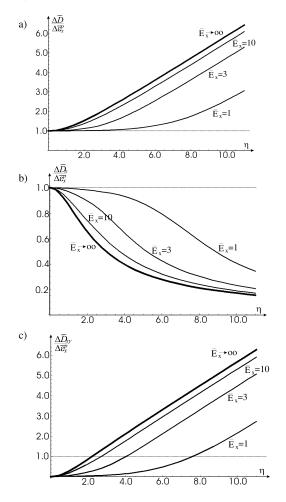
FIG. 12. a) Variation of the ratio of total plastic dissipation increment per cycle and the axial plastic strain increment (expense coefficient  $\delta$ ) with  $E_x$  and  $\eta$ , b) variation of axial expense coefficient c)variation of torsional expense coefficient.
