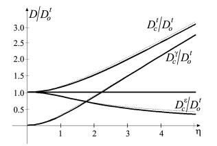
FIG. 4. Variation of the dissipated energy in one deformation cycle with the strain rate ratio  $\eta$ : continuous line – piecewise linear strain control, dashed line – harmonic shear strain control.
