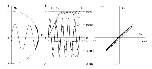
FIG. 15. Harmonic shear strain control with no maximal axial stress reduction and plastic response ( $\eta = 6$ ,  $\gamma_m/\varepsilon_0 = 0.924$ ) a) cyclic stress path, b) variation of axial and shear stress and shear strain, c) torsional hysteresis loop.
