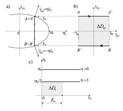
FIG. 2. Piecewise linear shear strain control: a) stress path, b) shear stress-strain hysteresis loop, c) axial stress variation.
