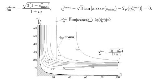
FIG. 8. Minimal values  $s_{\text{max}}$  of the tensile stress in the plane of process parameters  $\eta$ ,  $\gamma_m$ . Bold lines separate the regimes  $\mathcal{A}$ ,  $\mathcal{B}$ ,  $\mathcal{C}$  ( $m = m_{Al} = 0.128$ ).
