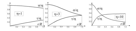
Fig. 19. Variation of axial stress and shear stresses in a cylinder for  $\eta = 1, 3, 10$ .
