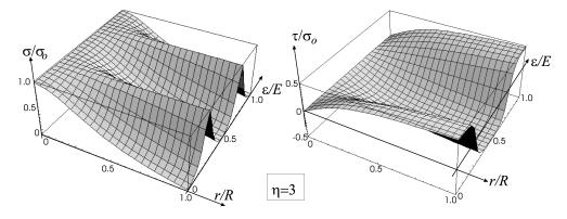
FIG. 22. The axial and shear stress distribution in cylinder for  $\eta = 3$ .
