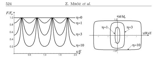
FIG. 23. Variation of axial force and twisting moment in the steady cyclic state for different values of  $\eta$ .
