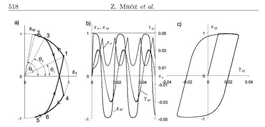
FIG. 13. Harmonic shear strain control with maximal axial stress reduction and elastoplastic response ( $\eta = 6$ ,  $\gamma_m/\varepsilon_0 = 4.62$ ) a) cyclic stress path, b) variation of axial and shear stress and shear strain, c) torsional hysteresis loop.
