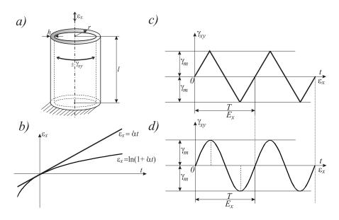
FIG. 1. Axial and torsional deformation program: a) tube dimensions, b) longitudinal strain  $\varepsilon_x(t)$ , c) piecewise linear variation of shear strain, d) harmonic variation of shear strain  $\gamma_{xy}(t)$ .
