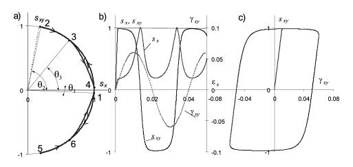
FIG. 14. Harmonic shear strain control with no maximal axial stress reduction and elastoplastic response ( $\eta = 6$ ,  $\gamma_m/\varepsilon_0 = 9.24$ ) a) cyclic stress path, b) variation of axial and shear stress and shear strain c) torsional hysteresis loop.
