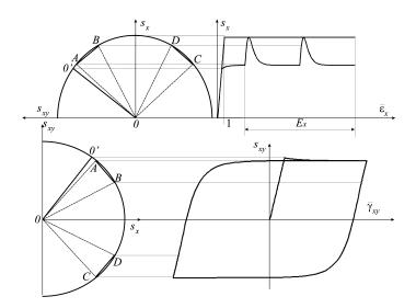
FIG. 10. Variation of the tensile stress path and the hysteresis loop of shear stress-strain response in the steady cyclic deformation,  $\eta_l < \eta < \eta_m$  regime  $\mathcal{B}$ : elastic unloading and no reduction of  $s_{\text{max}}$ .
