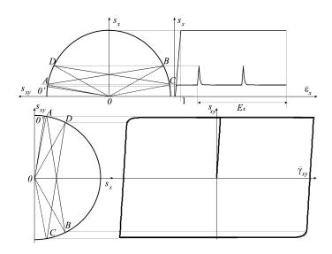
FIG. 11. Variation of the tensile stress path and the hysteresis loop of shear stress-strain response in the steady cyclic deformation,  $\eta > \eta_m$  (regime C: elastic unloading, maximal tensile stress reduction).
