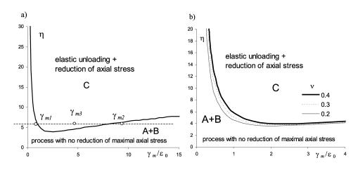
FIG. 16. The response diagram in the plane  $\gamma_m/\varepsilon_0$ ,  $\eta$  specifying domains  $\mathcal{A} + \mathcal{B}$  and  $\mathcal{C}$  of no-reduction and reduction of maximal axial stress a) diagram for large values of  $\gamma_m/\varepsilon_0$ , b) diagram for small values of  $\gamma_m/\varepsilon_0$ .
