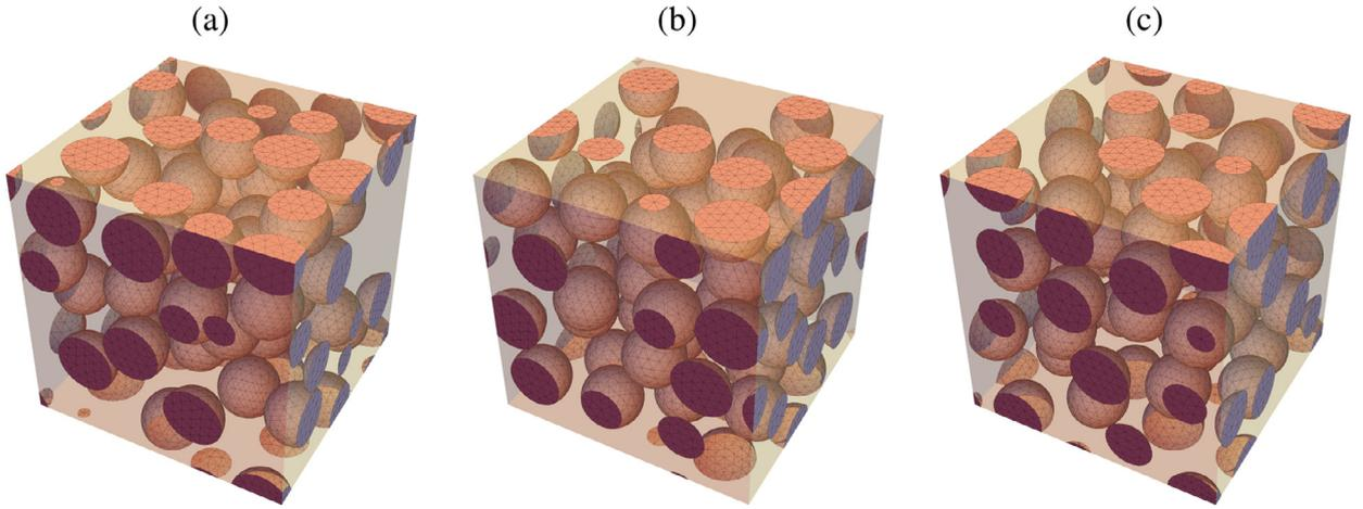
**Fig. 3.** Examples of periodic RVEs with 50 randomly-placed inclusions occupying a volume fraction  $f_i = 0.3$  (only the FE mesh of the inclusion phase is shown): a)  $\bar{\lambda}/(2R_i) = 0.039$ , b)  $\bar{\lambda}/(2R_i) = 0.164$ , and c)  $\bar{\lambda}/(2R_i) = 0.260$ .
