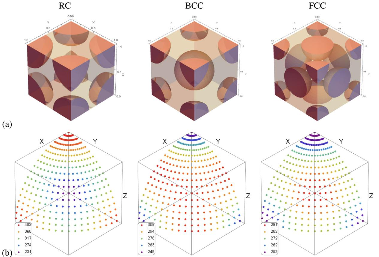
**Fig. 5.** (a) A view, in the (1,1,1) direction, of the RC, BCC, and FCC unit cells with  $f_i = 40\%$ . (b) Huber-von Mises equivalent stress  $\sigma_{Mises}$  [MPa] for  $\varepsilon = 3\%$  in the metal matrix composite undergoing a macroscopic tension test in a given direction  $\mathbf{v}$  (Eq. (17)). The viewing direction is (1,1,1); due to the symmetry of the results, only single octants are presented.
