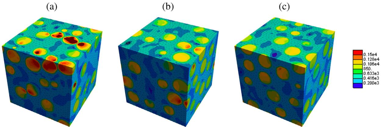
**Fig. 10.** Contour maps of the Huber-von Mises equivalent stress for the isochoric tension test at the strain  $\varepsilon = 3\%$  for the MMC composite with 50 spherical inclusions and  $f_i = 30\%$  (Fig. 3). The packing parameter  $\lambda/(2R_i)$  is equal to: (a) 0.039, (b) 0.164, (c) 0.260. Only the FE mesh of the matrix phase is shown.
