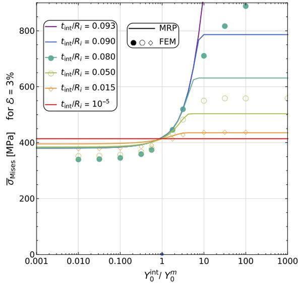
**Fig. 9.** The size effect for the RC arrangement of elastic inclusions in the metal matrix composite in the uniaxial strain test  $E_{(0,0,1)}$  (Eq. (18)) - Huber-von Mises equivalent stress at the strain  $\varepsilon = 3\%$  vs. relative yield stress of the interphase  $Y_0^{int}/Y_0^m$ . The size parameter  $t_{int}/R_i$  takes values according to the plot legend. The numerical results by FEM are presented as marks, while the MRP estimates as lines.
