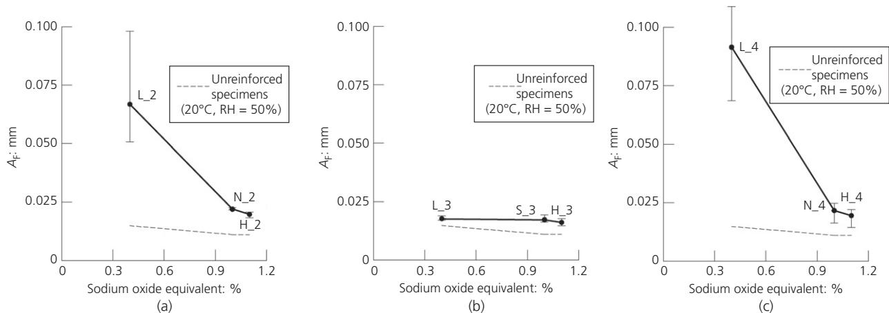
**Figure 10.** Area  $A_F$  measured in three-point bending tests: (a) specimens cured for 27 days in room conditions (20°C, RH = 50%); (b) specimens cured for 27 days in water (20°C); (c) specimens cured for 3 days in water (20°C)
