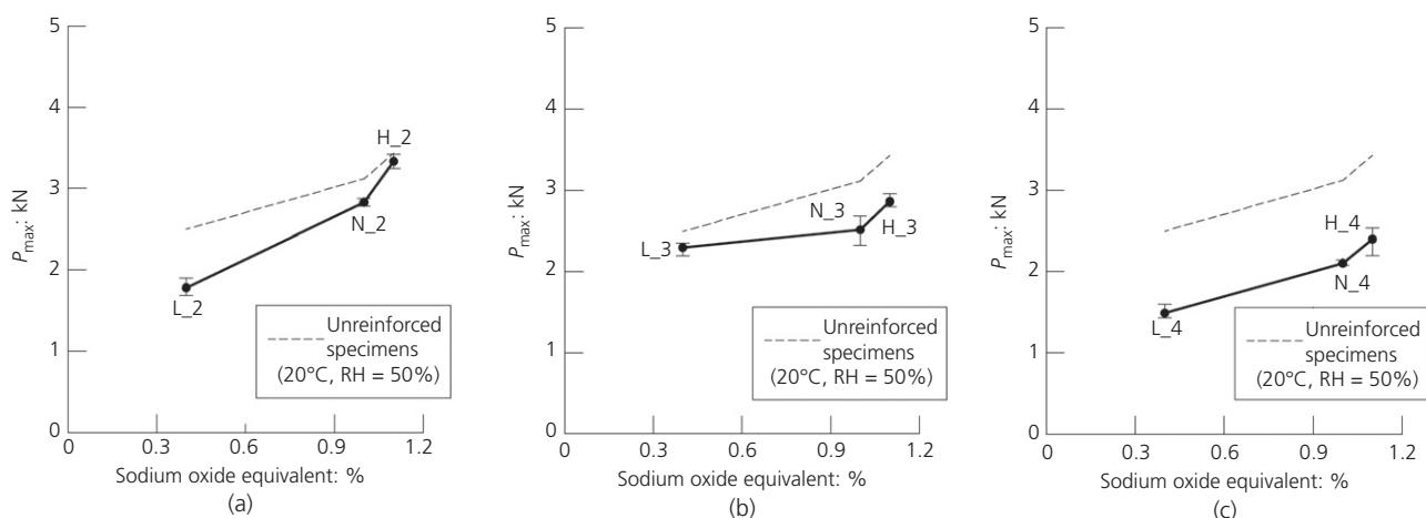
Figure 5. Flexural strength  $P_{max}$  measured in the three-point bending tests: (a) specimens cured for 27 days in room conditions ( $20^{\circ}\text{C}$ , RH = 50%); (b) specimens cured for 27 days in water ( $20^{\circ}\text{C}$ ); (c) specimens cured for 3 days in water ( $20^{\circ}\text{C}$ )
