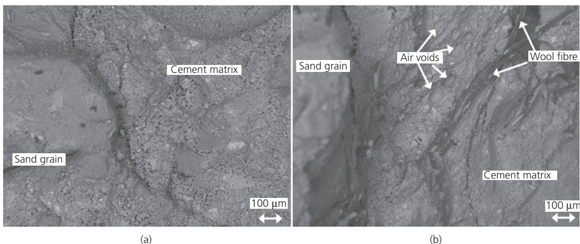
Figure 6. Microstructure of specimens made with low-alkali cement after 27 days of curing in  $20^{\circ}\text{C}$  and 50% RH (scale bar – 100  $\mu\text{m}$ ): (a) reference specimen L\_1; (b) specimen with addition of wool fibres L\_2
