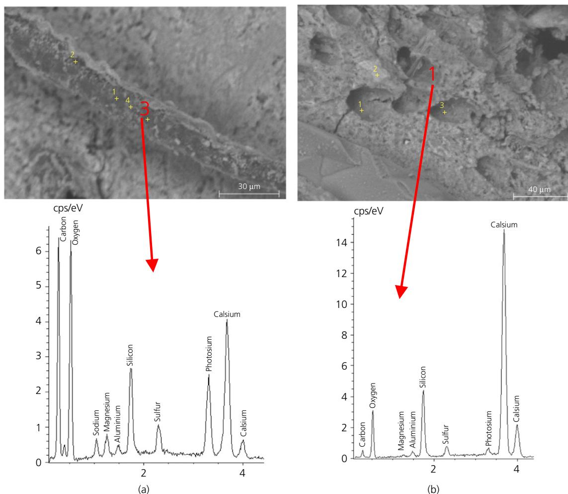
**Figure 7.** Microstructure of specimens made with high-alkali cement and reinforced with wool fibres with EDX analysis in microareas: (a) H\_4 – after 3 days of curing in water at 20°C (analysis in the microarea on a wool fiber); (b) H\_3 – after 27 days of curing in water at 20°C (microarea analysis in a matrix after a degraded wool fiber)
