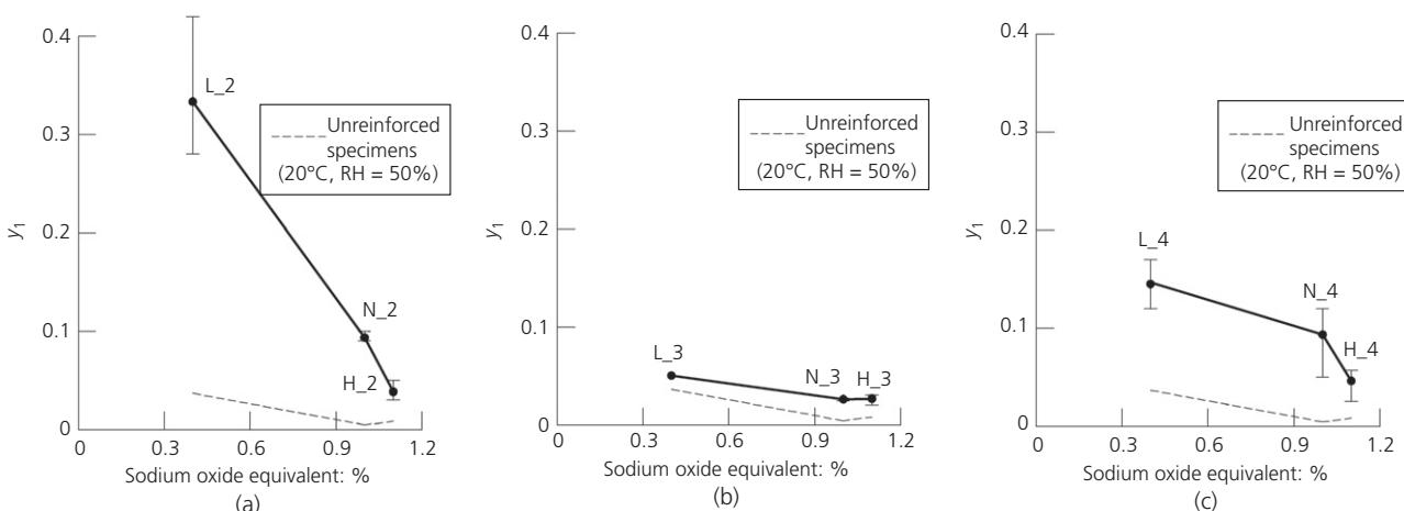
Figure 8. Residual stress  $y_1$  measured in the three-point bending tests: (a) specimens cured for 27 days in room conditions (20°C, RH = 50%); (b) specimens cured for 27 days in water (20°C); (c) specimens cured for 3 days in water (20°C)
