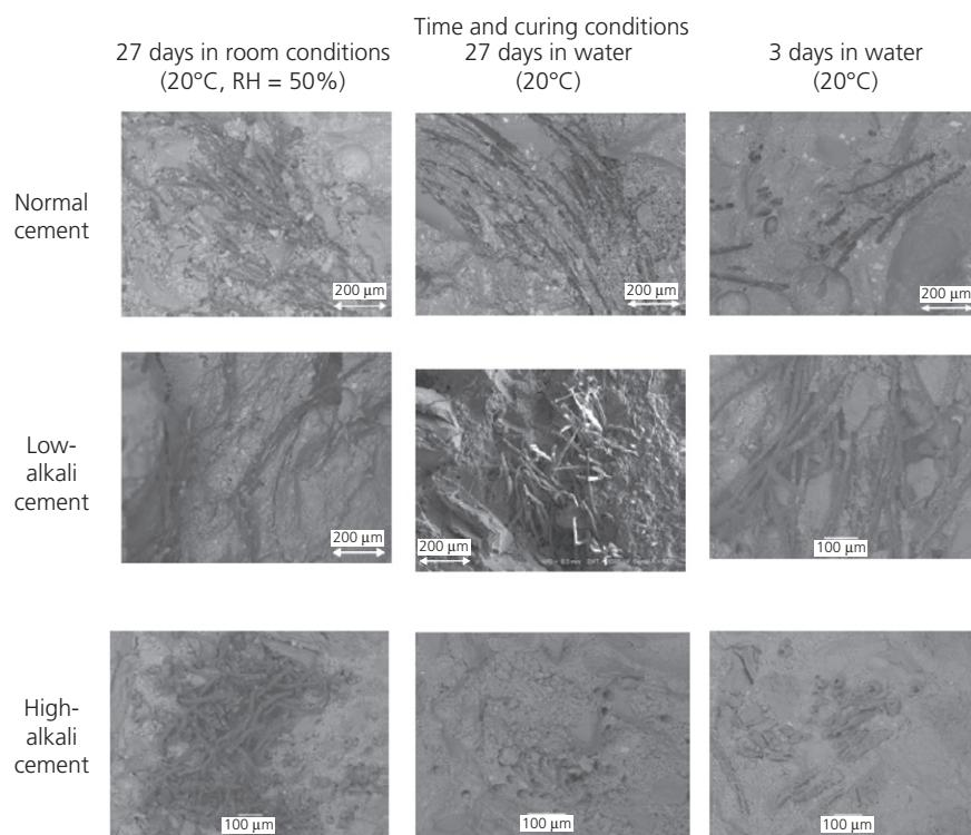
Figure 4. SEM images of the analysed mortars
