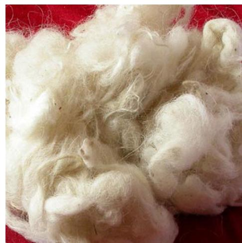
**Figure 1.** Sheep's wool used to reinforce cement-based mortars
