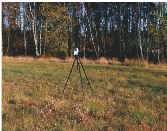
Fig. 8. On the left: the professional sound level meter SVAN 912A for measuring environmental noise placed on a tripod during operation at the point D. Top right: eight values (in dB(A)) of A-weighted equivalent sound level ( L_{Aeq} ) measured at points A–H and interpolated over the entire building plot. Bottom right: the stream plot of the gradient of L_{Aeq} .
