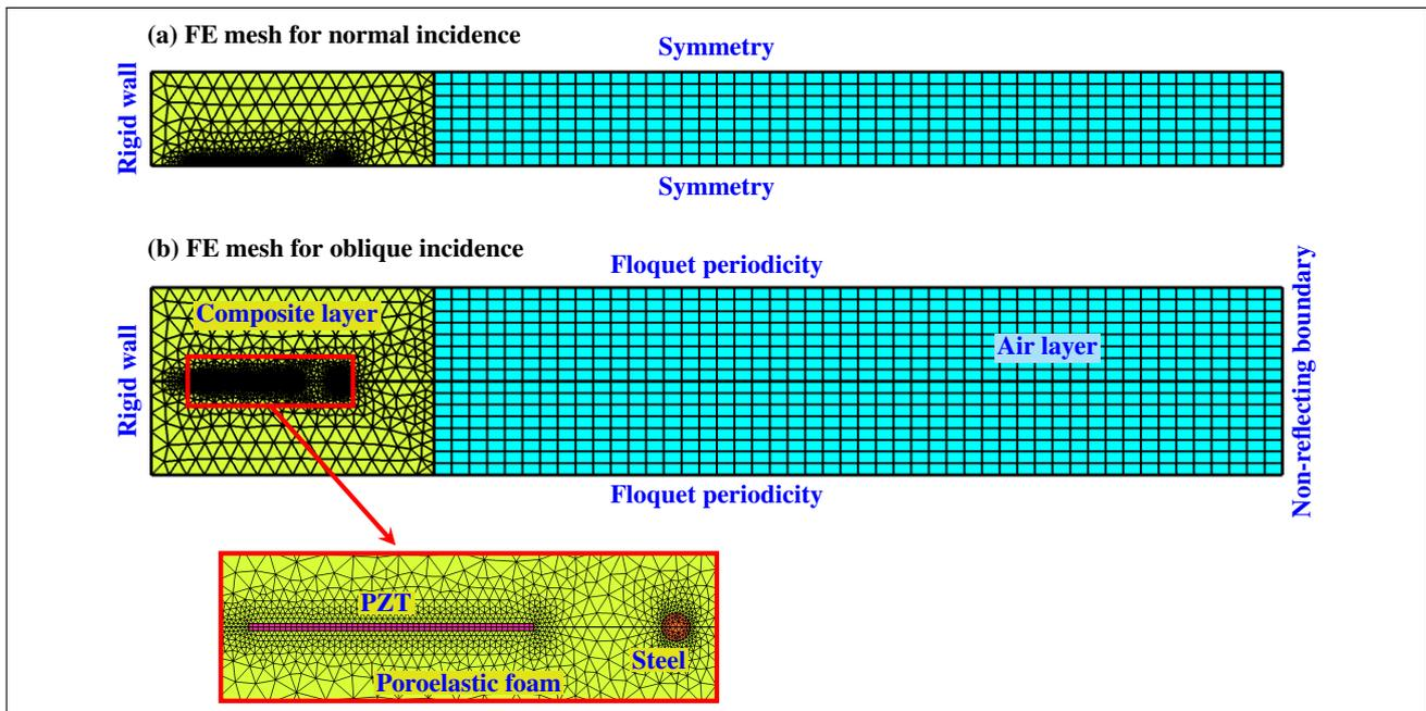
**Figure 1.** Problem configuration, boundary conditions, and finite-element meshes used for: (a) normal incidence, and (b) oblique incidence of plane harmonic waves.
