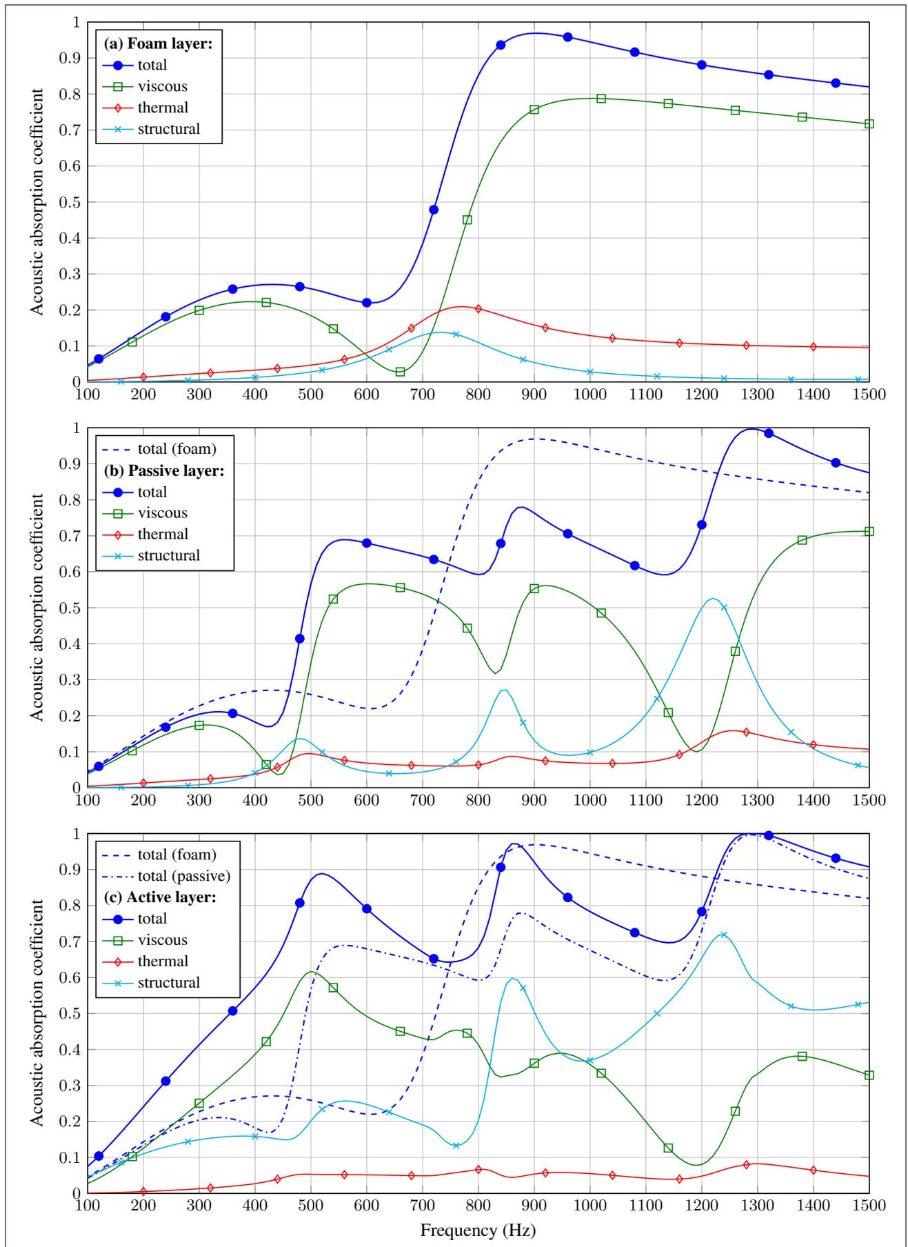
**Figure 3.** Total and partial acoustic absorptions at normal incidence for: (a) homogeneous poroelastic foam layer, (b) passive layer of poroelastic composite, (c) active layer of poroelastic composite.
