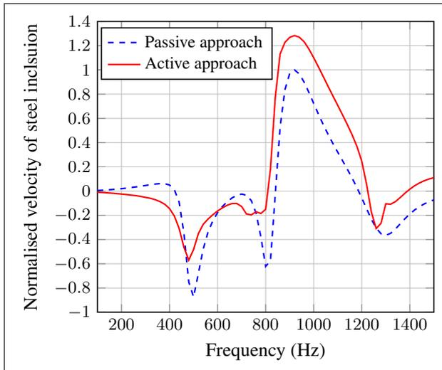
**Figure 5.** Normalized (dimensionless) velocity of the steel inclusion in the case of the passive and active approach.
