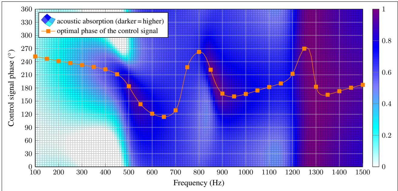
**Figure 4.** Optimised phase of the most effective control signal (with voltage amplitude of 60 V) acting on the PZT inclusion.
