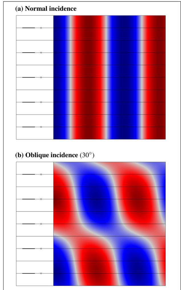
**Figure 2.** Acoustic pressure field (real part) in the adjacent air layer at 6 kHz for: (a) normal incidence and (b) oblique incidence ( $30^\circ$  from the normal direction) of plane waves.
